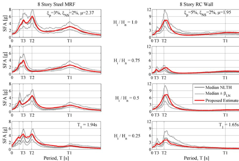
Fig. 5 – Comparison of proposed method with NLTH analysis at quarter points along the elevation with 2% nonstructural damping: 8 story steel MRF (left), 8 story RC wall (right). Median ductility demands are annotated
