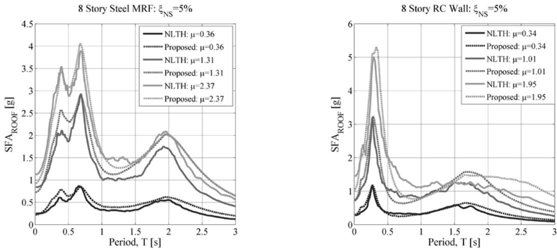
Fig. 7 – Comparison of proposed method with NLTH analysis at varying levels of ductility demand with 5% nonstructural damping: 8 story steel MRF (left), 8 story RC wall (right)
