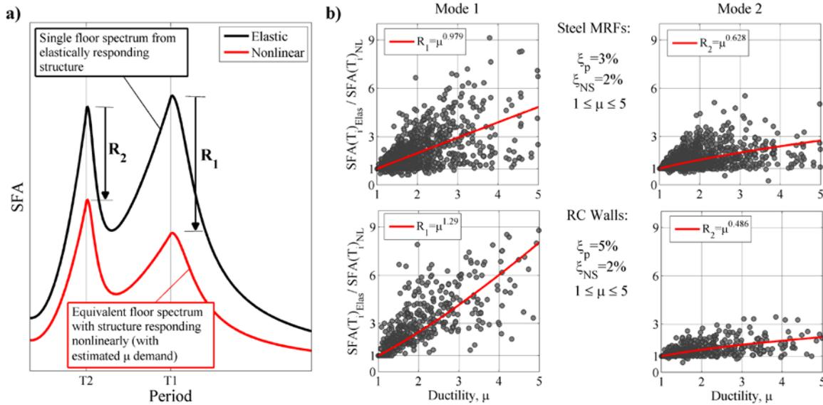
Fig. 4 – a) Definition of floor response spectrum (FRS) nonlinear reduction factors; b) Regression results for steel MRF buildings (above) and RC walls (below) for the first two modes at 2% nonstructural damping
