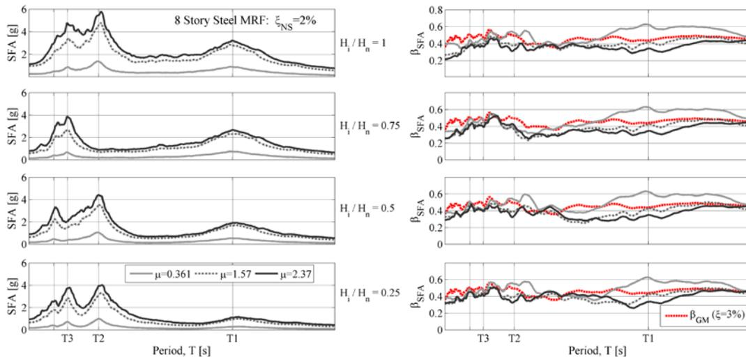
Fig. 8 – Median floor spectra from NLTH analysis for the 8 story steel MRF at various ductility demands 2%  $\xi_{NS}$  (left), corresponding lognormal dispersion compared with that of input ground motions (right)
