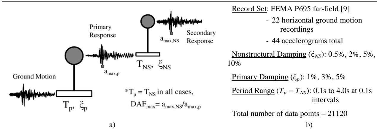
Fig. 2– Details of SDOF study for dynamic amplification: a) definition of  $DAF_{max}$ ; b) Input parameters
