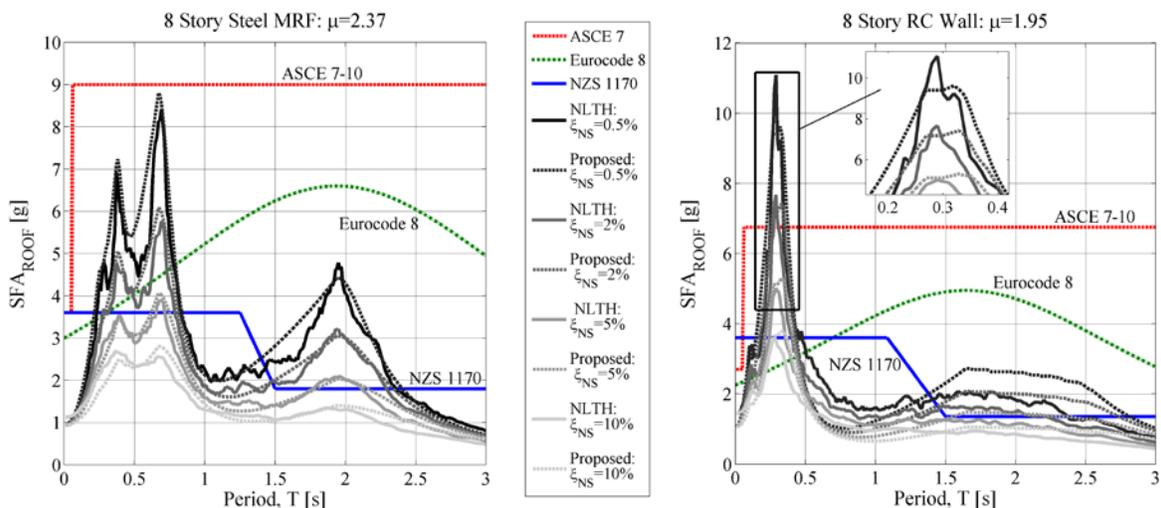
Fig. 6 – Comparison of proposed method with NLTH analysis at roof level for various values of nonstructural damping: 8 story steel MRF (left), 8 story RC wall (right). Current code approximations are annotated
