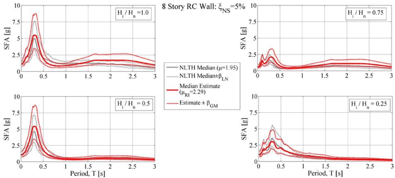
Fig. 11 – Estimates of dispersion compared with NLTH analysis using the dispersion of the input ground motion for the 8 story RC wall building at 5% nonstructural damping
