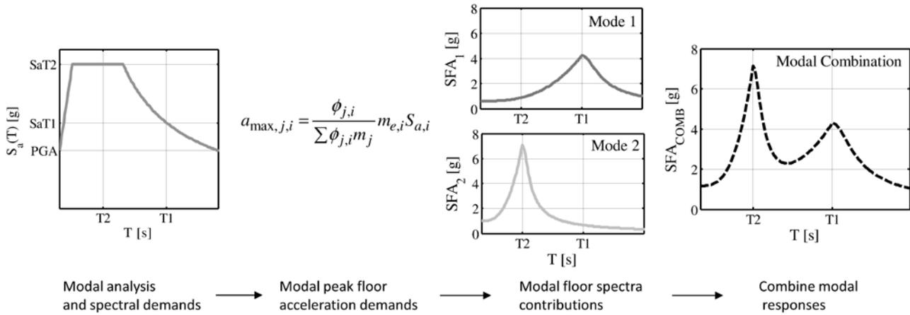
Fig. 1– Illustration of modal superposition for estimating floor response spectra
