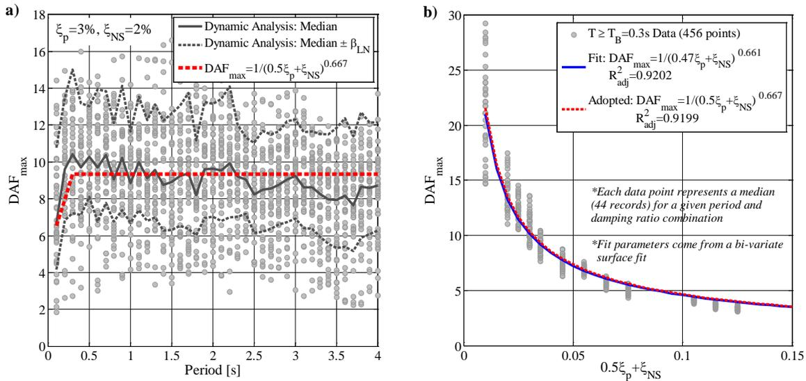
Fig. 3 – Adopted  $DAF_{max}$  function compared with median dynamic analysis results: a) Single damping ratio combination; b) All damping ratio combinations across all periods  $\geq T_B = 0.3s$ , with best fit and adopted equations indicated
