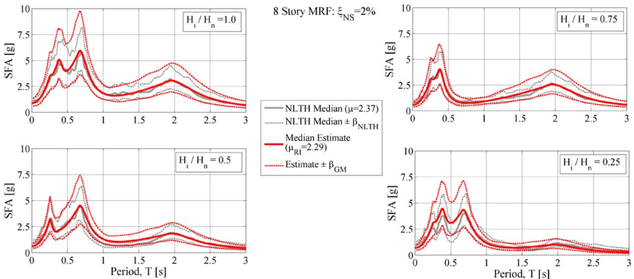
Fig. 10 – Estimates of median and dispersion compared with NLTH analysis using the dispersion of the input ground motion for the 8 story steel MRF building at 2% nonstructural damping
