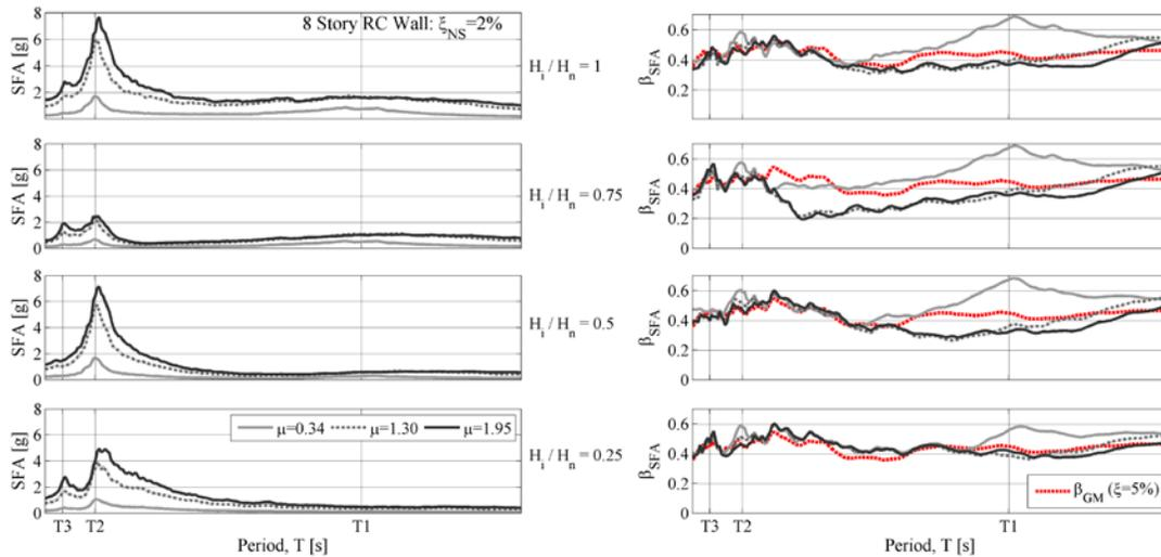
Fig. 9 – Median floor spectra from NLTH analysis for the 8 story RC wall at various ductility demands 2%  $\zeta_{NS}$  (left), corresponding lognormal dispersion compared with that of input ground motions (right)
