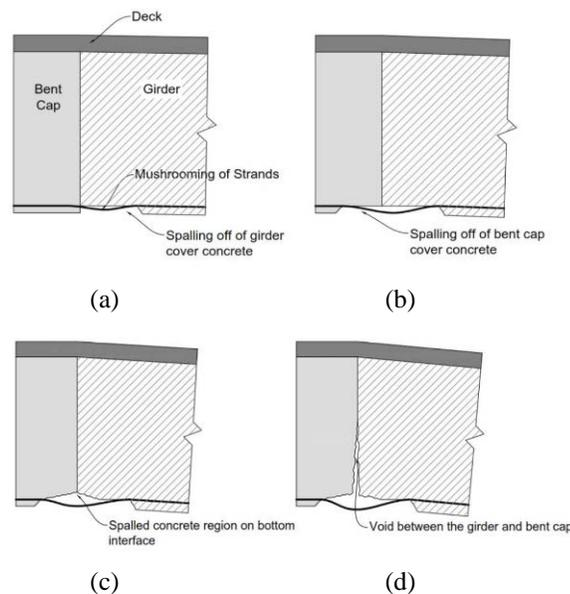
Fig. 6 – Illustrations showing Softening of Negative Moment Resistance
