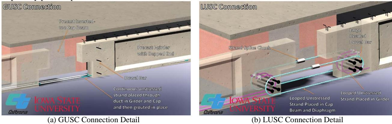
Fig. 1 – Schematic of Two Connections used between Precast I-shaped Girders and Precast Inverted-tee Cap Beam
