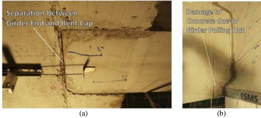
Fig. 7 – Damage Resulting from Mobilizing the Shear Friction Mechanism
