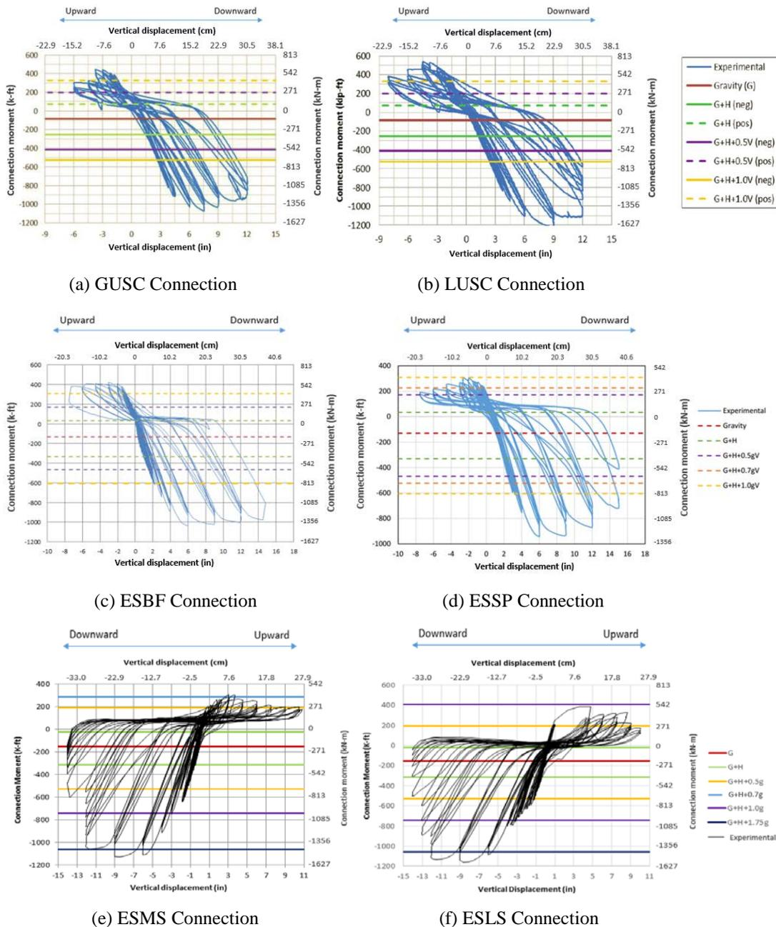
Fig. 5 – Measured Connection Moment as a Function of Displacement of Actuator 2
