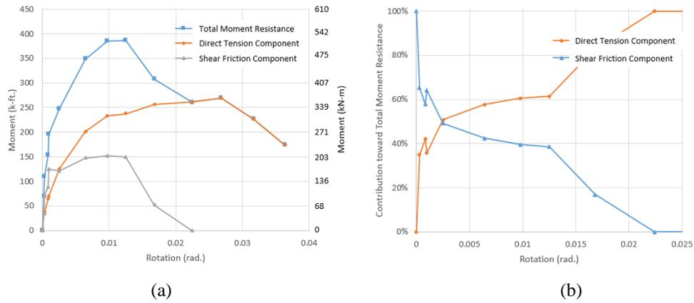
Fig. 9 – Moment Contributions and Percentages of Positive Moment Resistance in ESLS Connection
