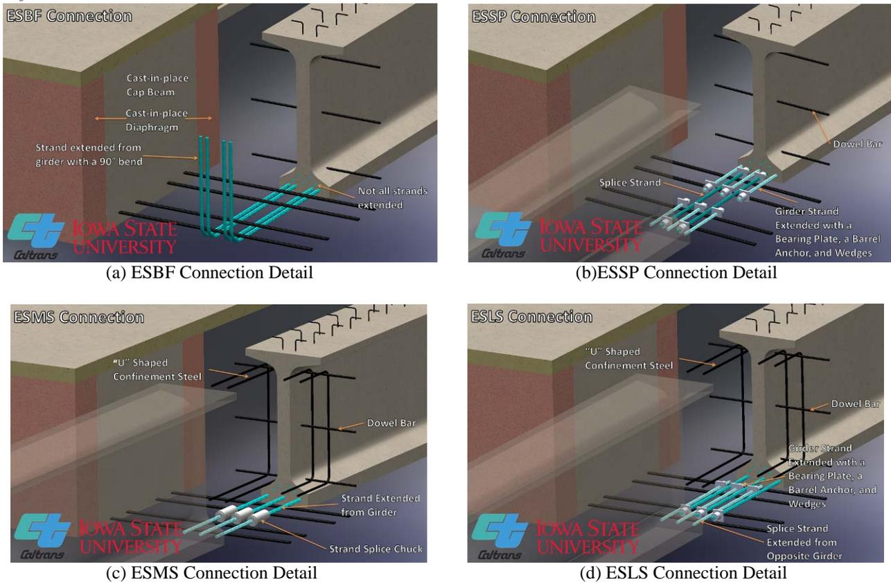
Fig. 2 – Schematic of Four Connections used between Precast Bulb-tee Girders and Cast-in-place Cap Beam
