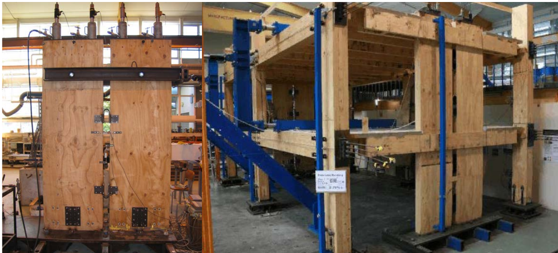
Fig. 4 - Coupled walls and two-storied building model [25, 27]
