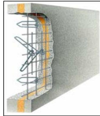
Fig. 2 – Concrete Sandwich Panel
