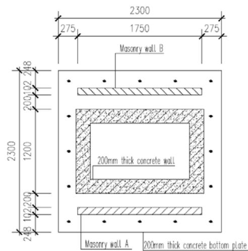
Fig. 8: Plan of test specimen
