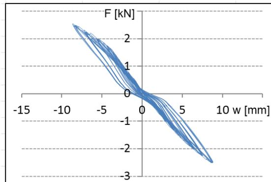
Fig. 25: anchor type 1 under alternating shear loading
