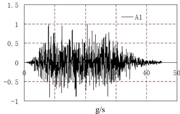
Fig. 15: Normalized time interval curve of artificial wave
