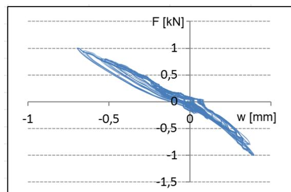
Fig. 27: anchor type 2 under pressure / tension load
