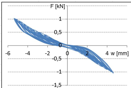
Fig. 26: anchor type 2 under alternating shear load
