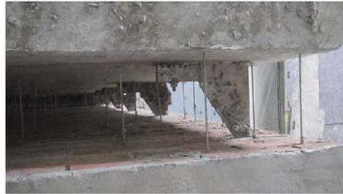
Fig. 19: Brackets and brick ties after test
