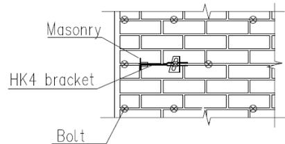
Fig. 11: Elevation of brick ties and horizontal HK4 bracket on masonry wall B      Fig. 12: Detail of brick ties and horizontal HK4 bracket on masonry wall B
