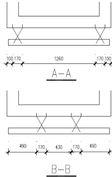
Fig. 9: Layout of brick ties on masonry wall A      Fig. 10: Sectional details of brick ties on masonry wall A
