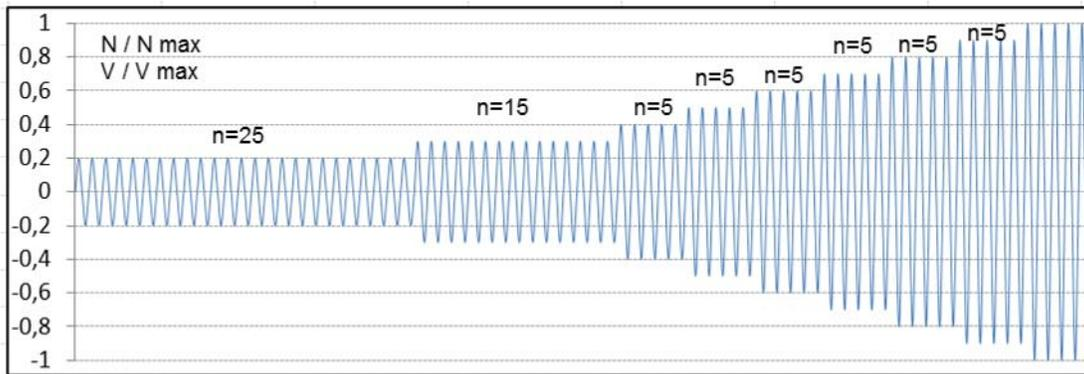
Fig. 24 – Load amplitudes for tests under pulsating pressure /tension load and alternating shear load
