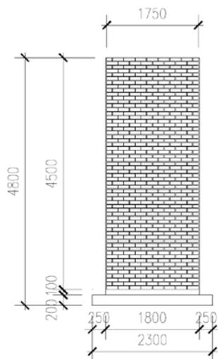
Fig. 7: Elevation of the test specimen
