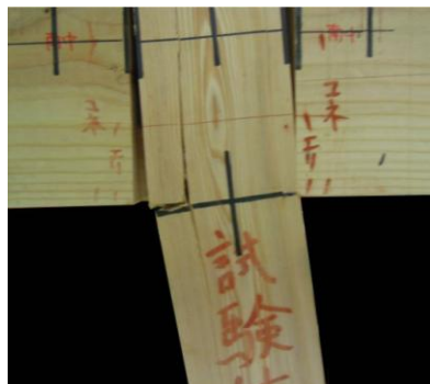
(a) Breakage of column (5P12-12-12f, Column Cl)
