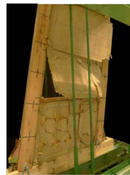
(b) Breakage of wall (5P12-12-12f, First story section)
