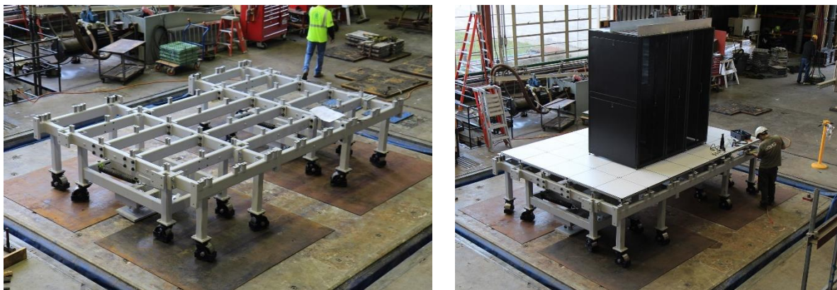
Fig. 6: Shake Table Testing of the Floor Isolation System at UC Berkeley: (a) Bare floor frame, and (b) Tile-stringer-pedestal system installed on top of the floor along with server racks
