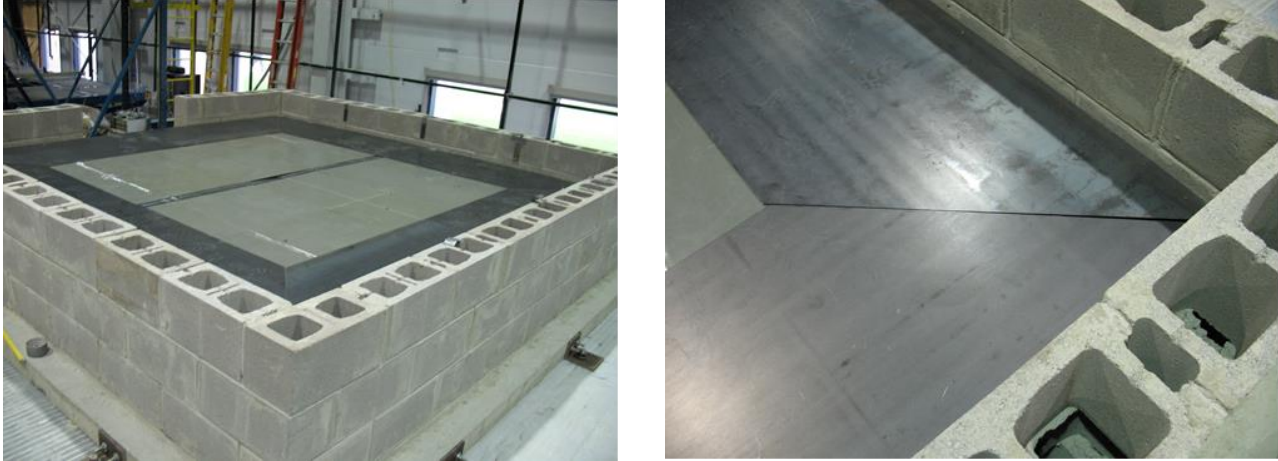
Fig. 5: (a) Overall View of the System tested at UB (lighter grey surface is the movable isolated floor; darker grey is the set of edge plates attached to the concrete wall); (b) Close-up of Corner Configuration of Edge Plates
