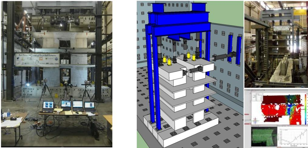
Fig. 7 Coupled shear wall test specimen with multi-directional loading, joint strains measured by DIC system
