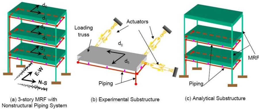
Fig. 5 – RTHS of 3-Story MRF with piping system subjected to bi-directional ground motions.
