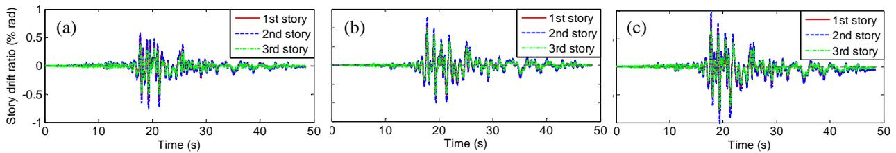
Fig. 9 Story drift ratio time histories from DBE level RTHS using HECTOR-11625090 record: (a) building designed for 100%, (b) 75%, and (c) 60% of the design base shear.
