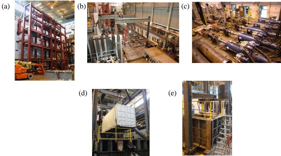
Fig. 3 – Lehigh NHERI EF testbeds: (a) lateral force resisting system testbed; (b) non-structural component multi-directional seismic simulator; (c) 5 full-scale damper testbeds; (d) tsunami debris impact force testbed; and, (e) soil boxes.
