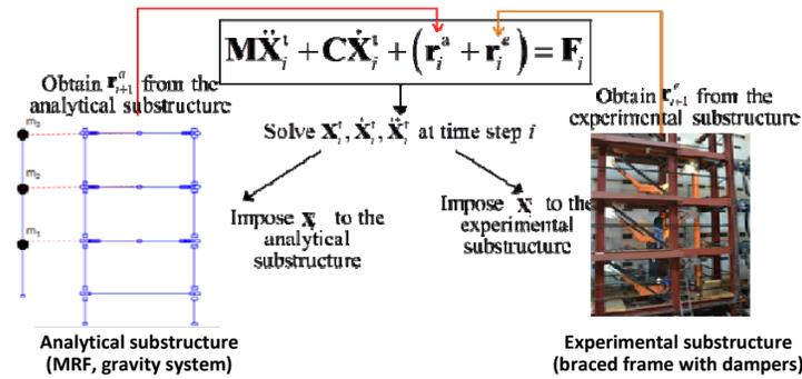
Fig. 8 Analytical and experimental substructures for RTHS of a 3-story building with nonlinear viscous dampers.
