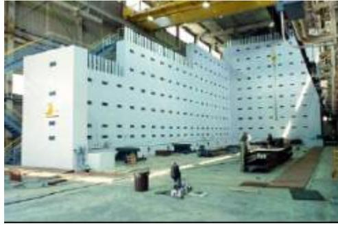
Fig. 1 – ATSS Laboratory Multidirectional Reaction Wall
