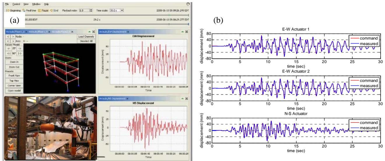
Fig. 6 – RTHS of 3-Story MRF with piping system: (a) teleobservation of animated system response, video of experimental substructure; and, (b) EW and NS 3<sup>rd</sup> floor displacements.
