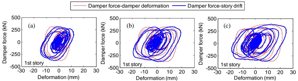
Fig. 10 Damper force-deformation responses from DBE level RTHS with HECTOR-11625090 record: (a) building designed for 100%, (b) 75%, and (c) 60% of the design base shear.
