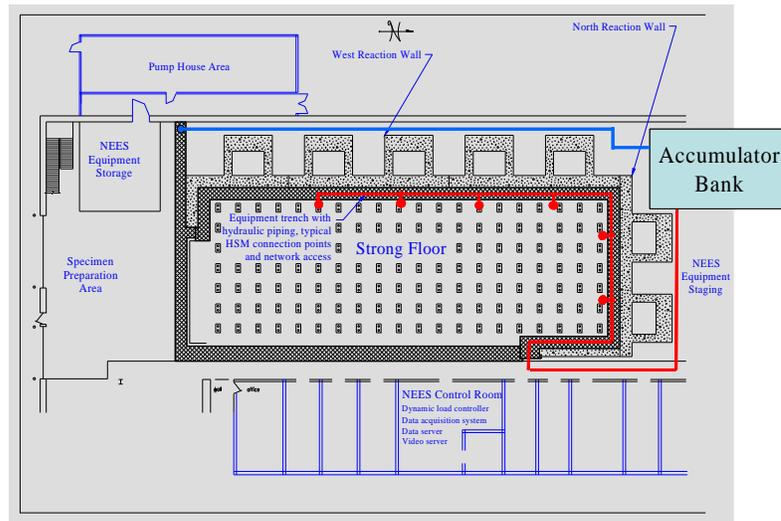
Fig. 2 – Floor Plan of ATSS Laboratory with Lehigh NHERI EF.
