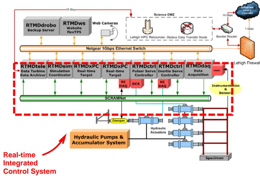
Fig. 4 – Lehigh NHERI EF Real-Time Integrated Control System.
