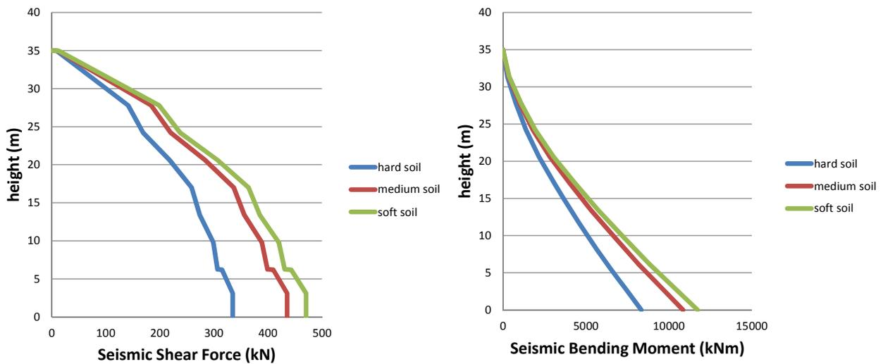
Figure 5. Distributions of seismic shear forces and bending moments for the tall towers in Indonesia (Seismic design code of SNI-02-01726-2002, Seismic zone 6, Importance factor = 1.0, Reduction factor (R) =2.9 (same as UBC))
