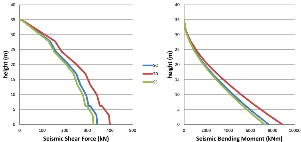
Figure 7. Distributions of seismic shear forces and bending moments for the tall towers in the Philippines (Seismic design code of NSCP 2010, Seismic zone 4)
