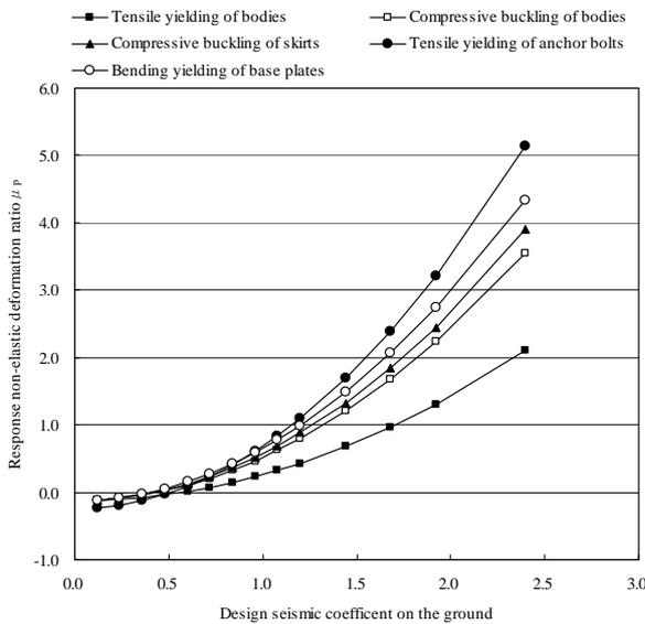
Figure 11. Relationship between design seismic coefficients on the ground (SCG) and nonelastic deformation ratios for towers
