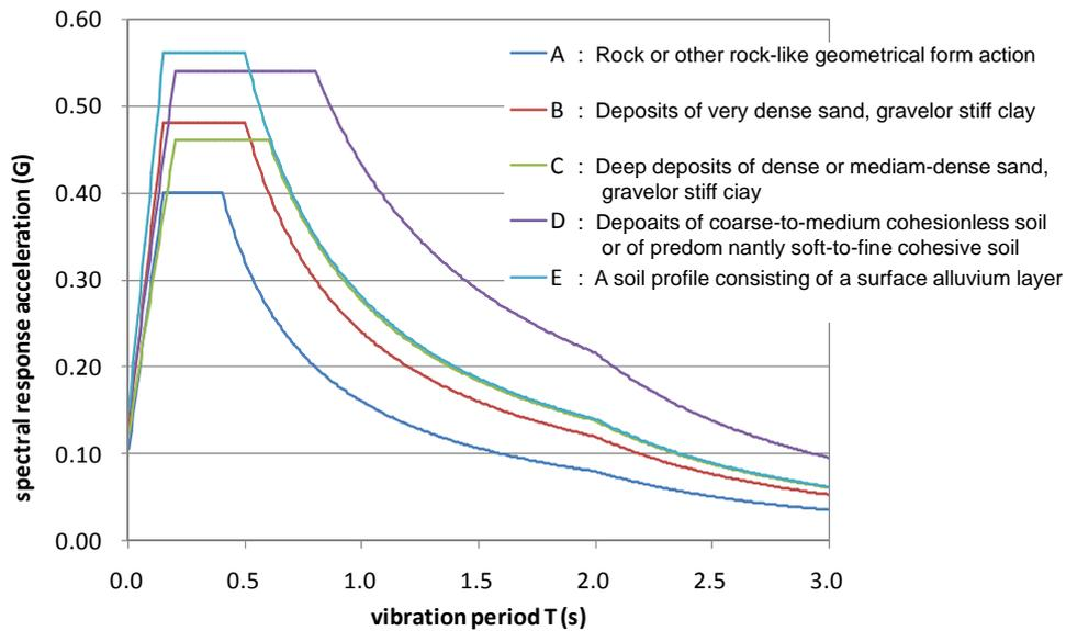
Figure 2. Horizontal elastic response spectra for earthquakes in Vietnam (Seismic design code of TCXDVN 375-2006, Peak ground acceleration = 0.16G, Importance factor = 1.0, Behavior factor = 1.0, Damping factor = 5%)
