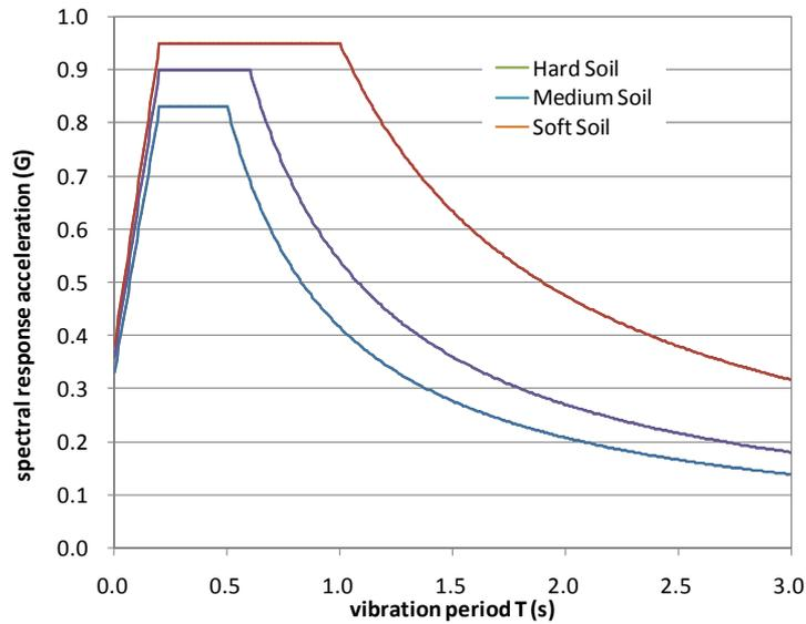
Figure 4. Horizontal elastic response spectra for earthquakes in Indonesia (Seismic design code of SNI-02-01726-2002, Seismic zone 6, Damping factor =5%)
