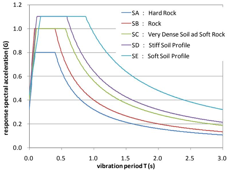
Figure 6. Horizontal elastic response spectra for earthquake in the Philippines (Seismic design code of NSCP 2010, Seismic zone 4, Damping factor = 5%)
