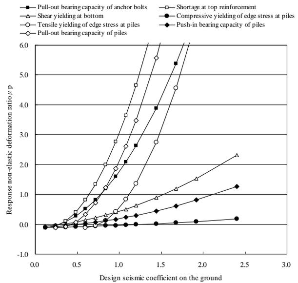
Figure 12. Relationship between design seismic coefficients on the ground (SCG) and nonelastic deformation ratios for foundations
