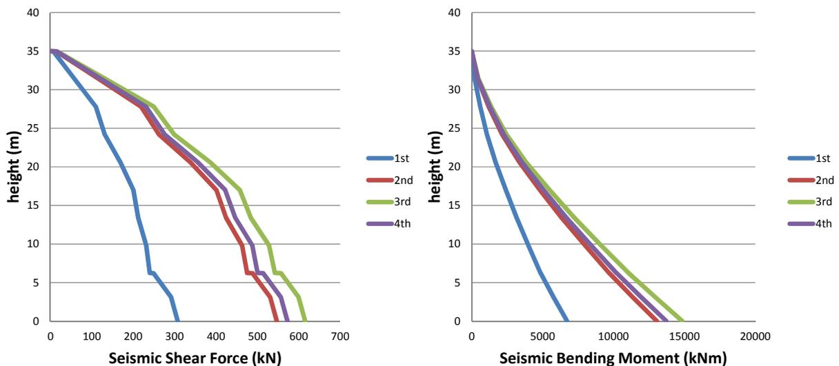
Figure 9. Distributions of seismic shear forces and bending moments for the tall towers in Japan (Seismic design code of HPGF-KHK, Importance factor =0.8, Zone SA)
