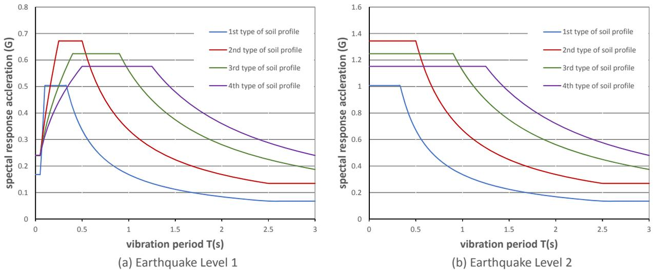
Figure 8. Horizontal elastic response spectra for earthquakes in Japan (Seismic design code of HPGF-KHK, Seismic importance class I, Zone SA, Damping factor = 5%)
