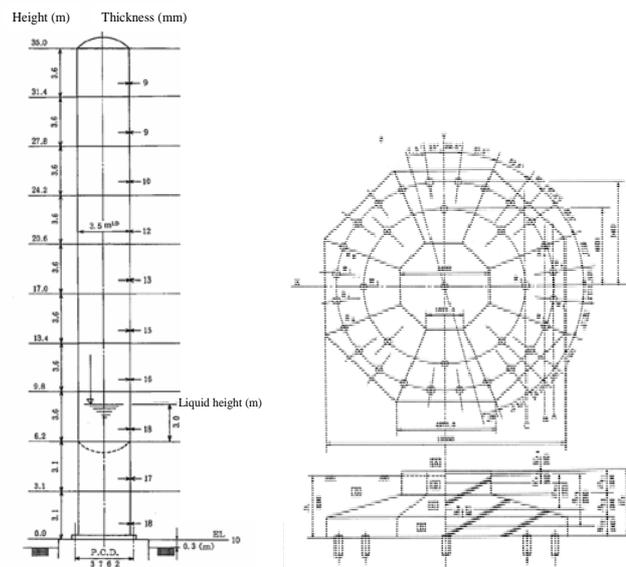
Figure 10. Calculation model for sensitivity analysis of a tall tower and the foundation
