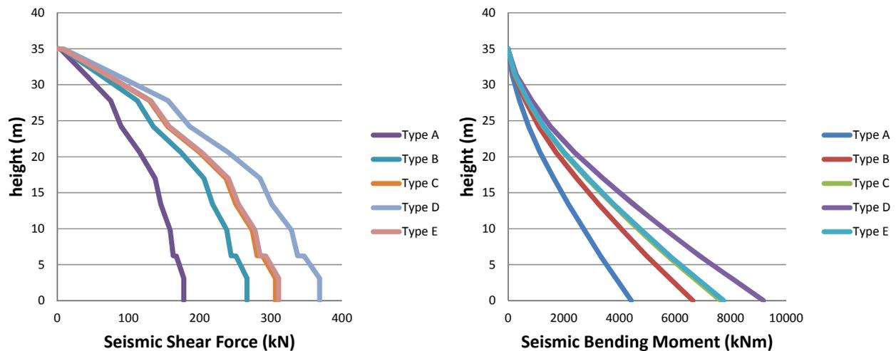
Figure 3. Distribution of seismic shear forces and bending moments for the tall tower in Vietnam (Seismic design code of TCXDVN 375-2006,  $a_g R = 0.16$ , Importance factor = 1.0, Behavior factor ( $q$ ) = 2.0)
