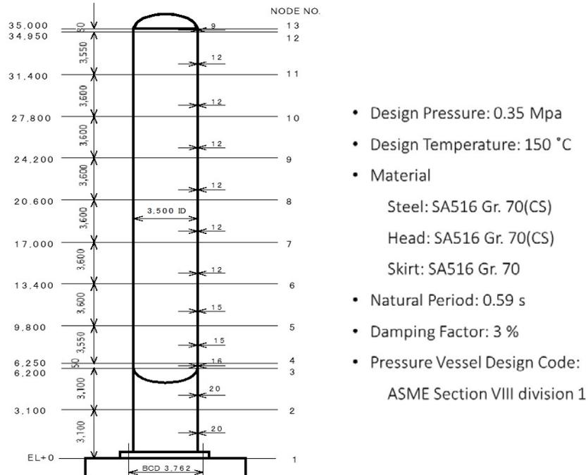
Figure-1 Calculation model for seismic design of a tall tower
