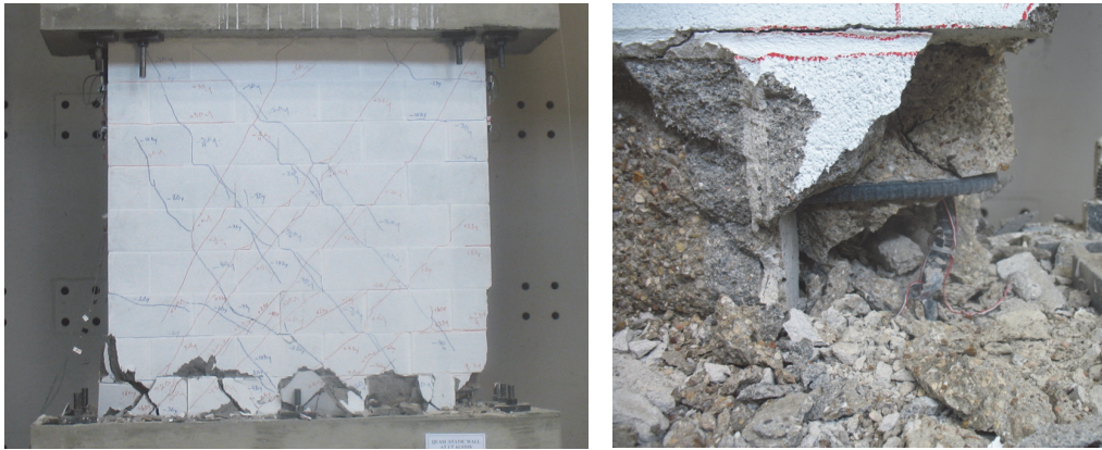
Fig. 2 – Final condition of the masonry wall, diagonal cracks crossing the field of the wall and sliding at the base (left) and toe crushing of the inferior right corner of the masonry wall (right) [3]
