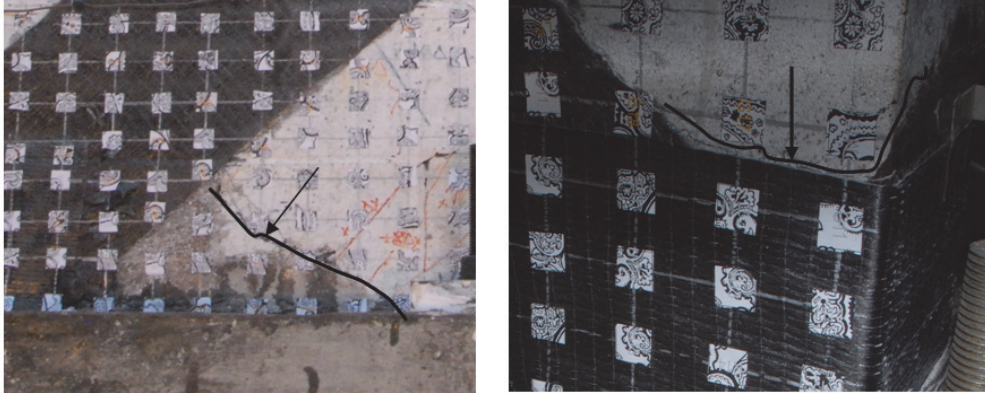
Fig. 8 – Existing cracks opened after reach maximum south (left) and north (right) lateral displacement.
