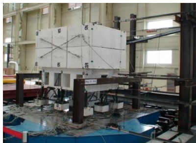
(a) Overview of earthquake simulation test set-up
