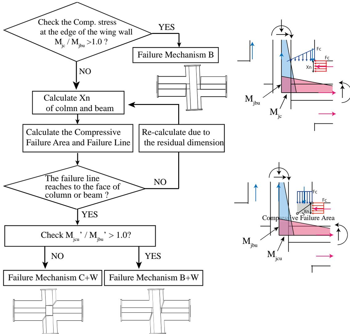
Fig. 3 –Flow chart of the proposed design procedure
