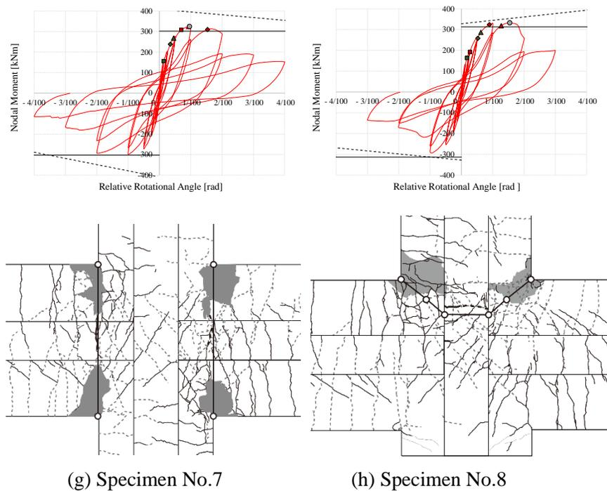
Fig. 4 –Relationship between nodal moment and rotational angle and crack pattern
