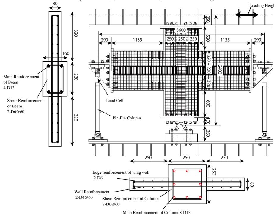
Fig. 1 – Example of bar arrangement (Specimen No.3)
