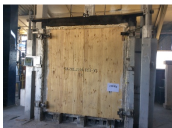
Figure 8 - Fire resistance test. Front view
