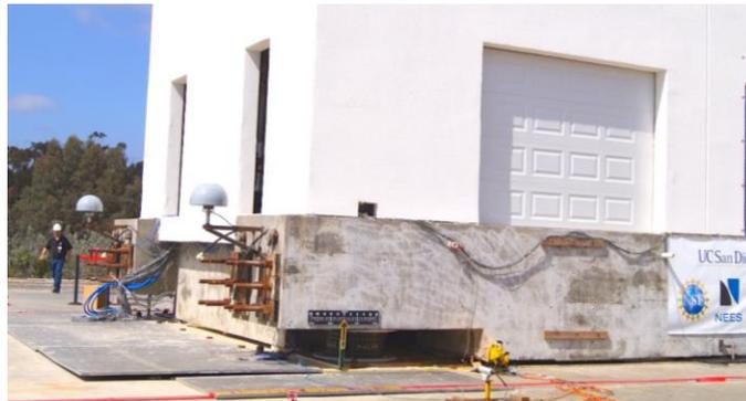
(c) Photo of bearing installed under building on shake table
