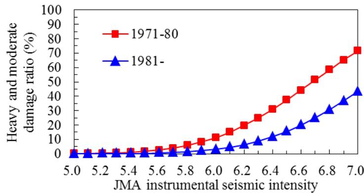
Fig. 3 - The fragility curves for non-wood-frame buildings
