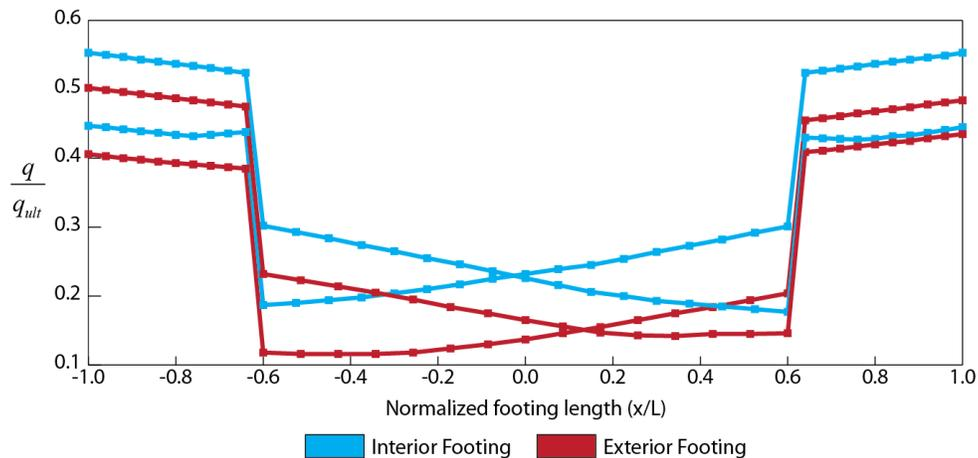
Fig. 8 – Median maximum normalized forces in springs for interior and exterior footings (site class D)
