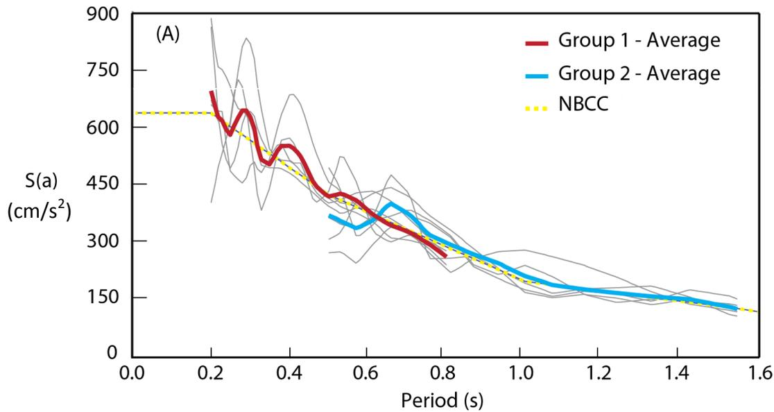
Fig. 2 – Comparison between the median spectra of the simulated ground motions for low-frequency and high-frequency record sets and the target NBCC (CODE) spectrum for class D site.
