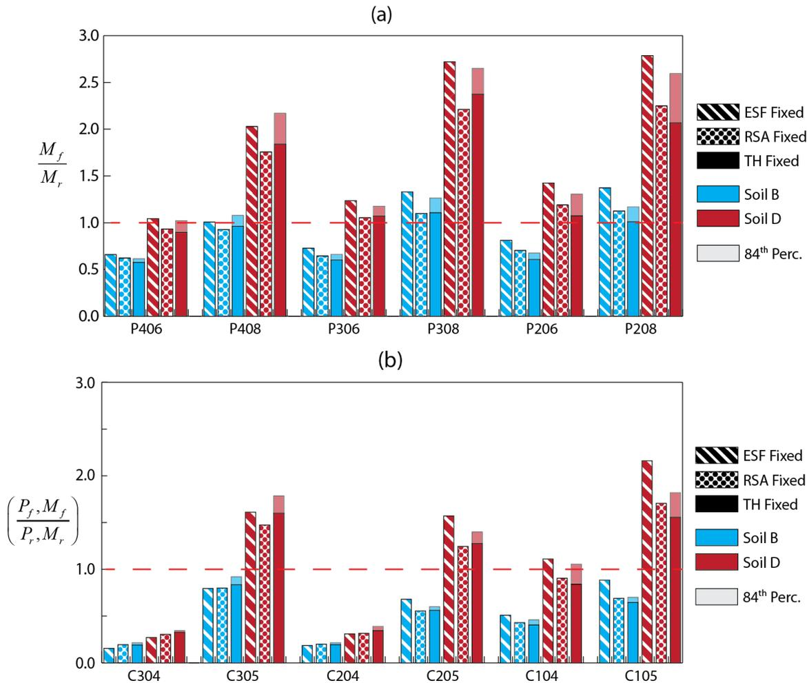
Fig. 4 – Fixed boundary conditions: Comparison of (a) beam end-moment demand-to-capacity ratio and (b) axial force-moment demand-to-capacity ratio for columns.
