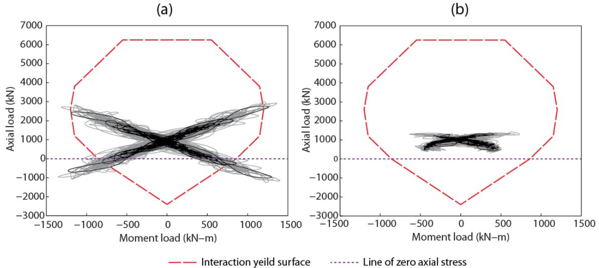
Fig. 6 – Site class D: Axial-force-moment demand of column C105 for (a) fixed boundary conditions and (b) flexible boundary conditions
