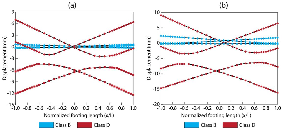
Fig. 7 – Median peak foundation uplift and soil settlement (a) exterior footings and (b) interior footings
