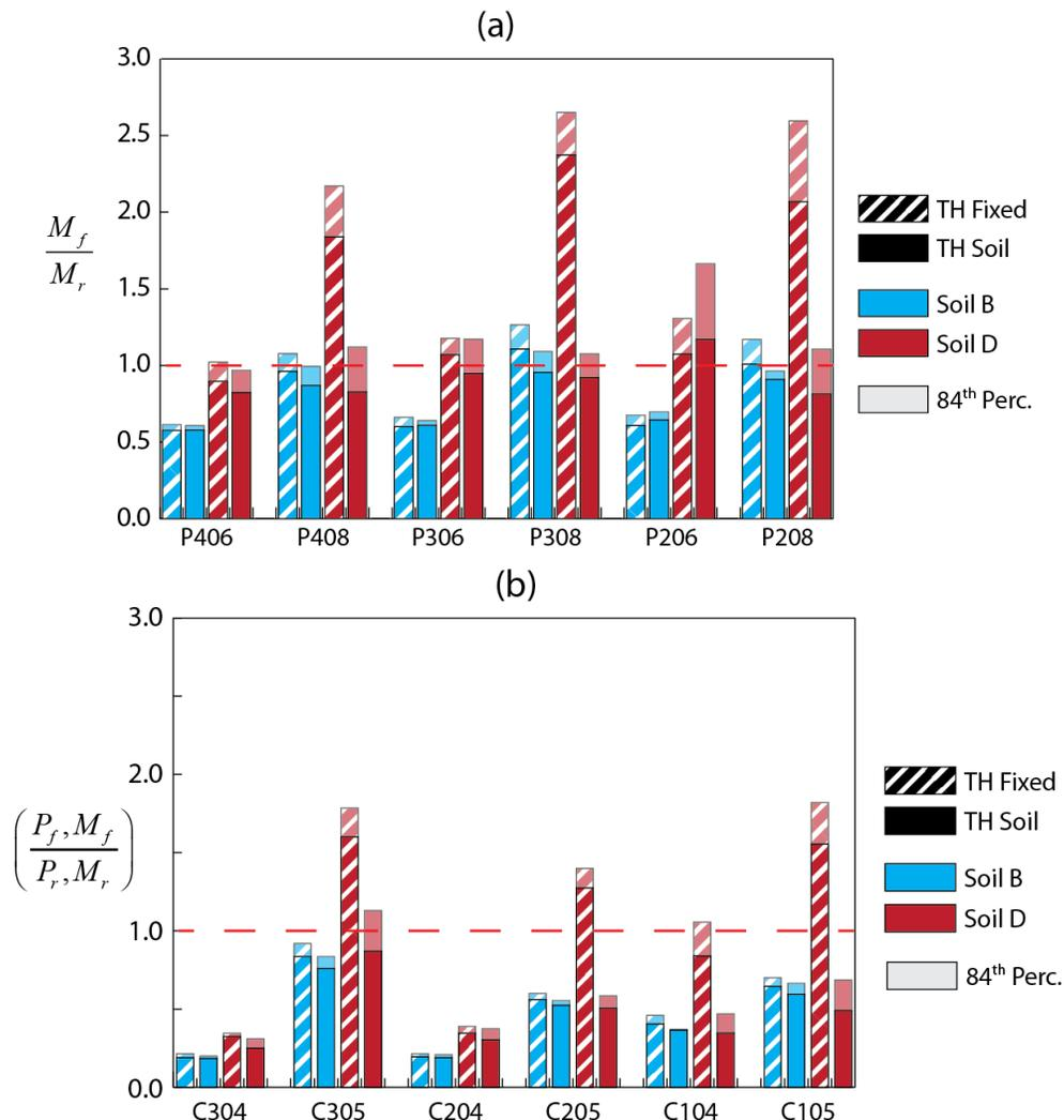
Fig. 5 – Comparison of (a) beam end-moment demand to capacity ratio and (b) axial-force-moment demand to capacity ratio for fixed and flexible boundary conditions.
