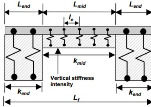
Fig. 3 – BNWF mesh discretization with variable stiffness ratio and end-length ratio.
