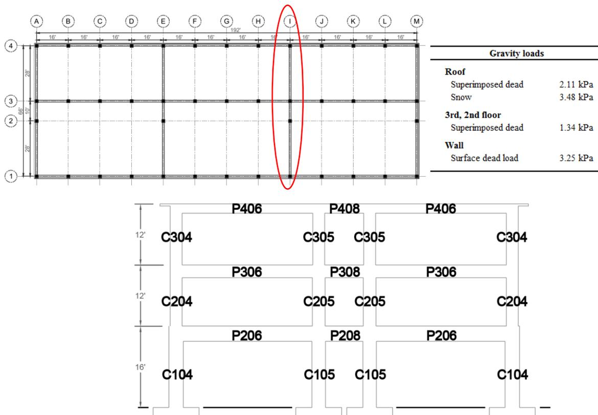
Fig. 1 –Typical floor plan, elevation and design gravity loads
