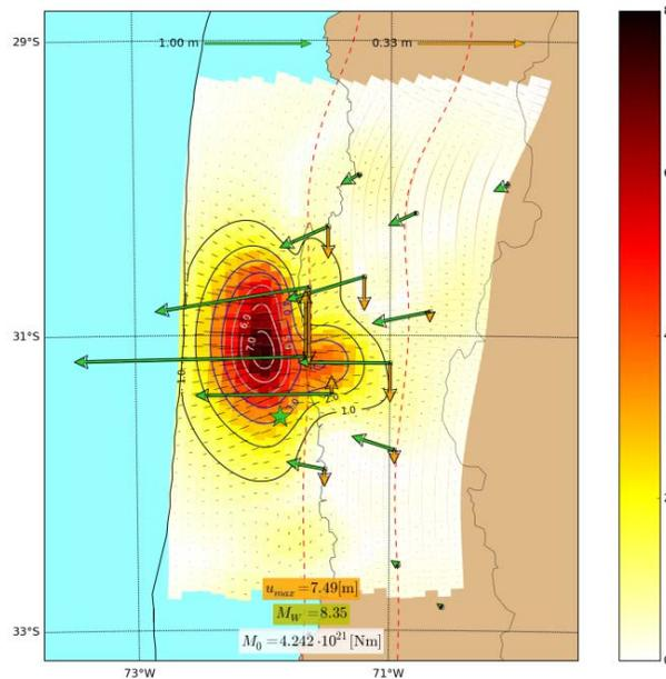
Fig. 4. Final (right) estimation of slip distribution of the 2015 Illapel earthquake from displacement data observed at the surface [10]. The first estimation was obtained after 33 hours of origin time. The goal is to diminish this number to few minutes, considering the source duration.
