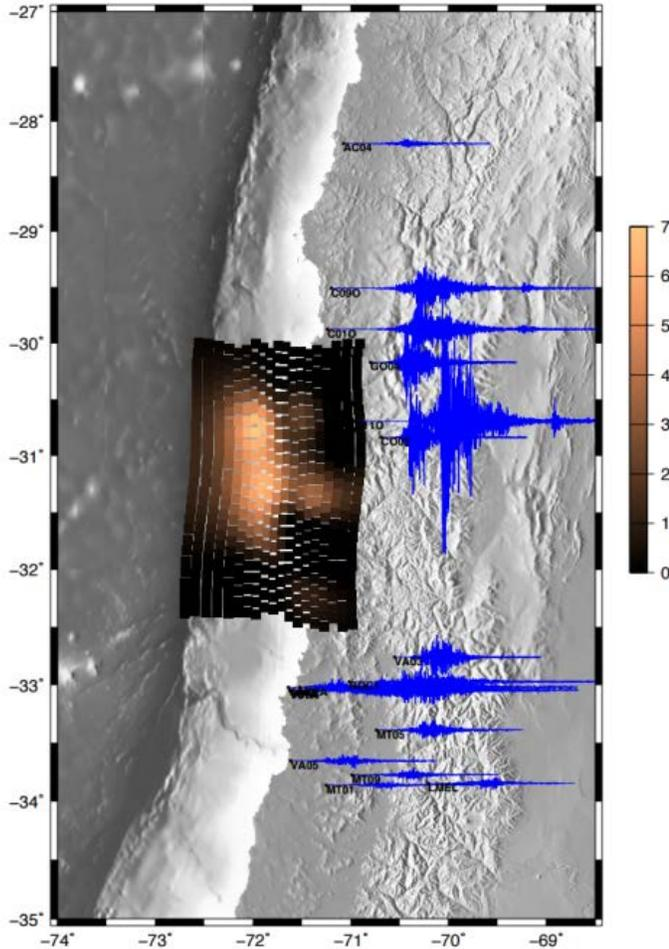
Fig. 5. Strong motion records associated with the 15 September (Mw=8.4) Illapel earthquake. Maximum accelerations of the order of 60%g were recorded at stations directly inland of the major displacement along the rupture plane (SLAB1.0 model, [13]).
