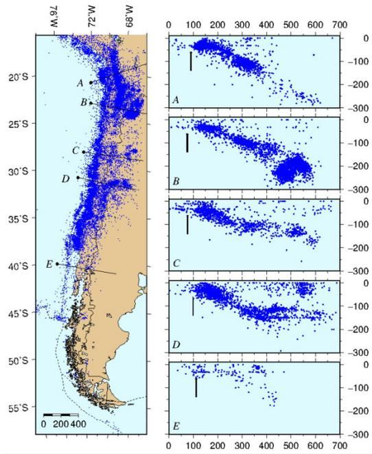
Fig. 1. Five profiles (right panels) show the depth distribution of earthquakes as a function of distance from the trench. The catalog includes three sources of information SISRA [5] (1900-1981), USGS (1982-1999), CSN (2000-2015)
