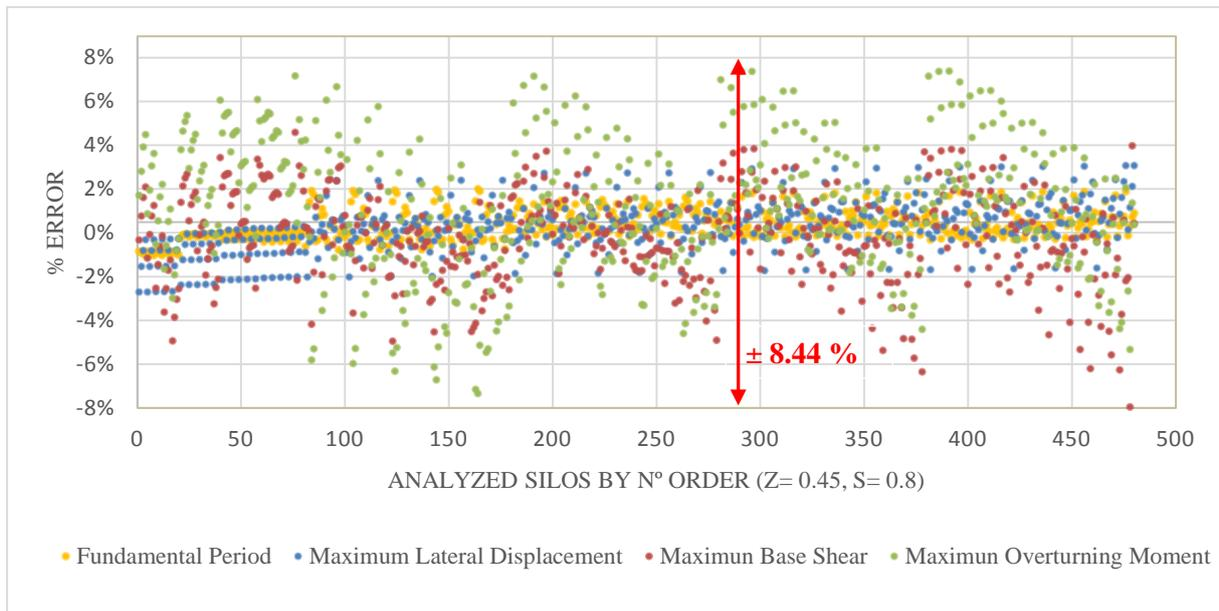
Figure 4. Percentage error of the different responses of the silos analyzed: simplified method versus spectral modal combination.
