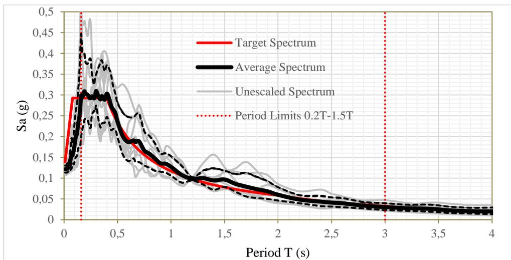
Figure 3. Pseudo-acceleration design spectrum: E030 [3] (red) and arithmetic mean of chosen records (black).
