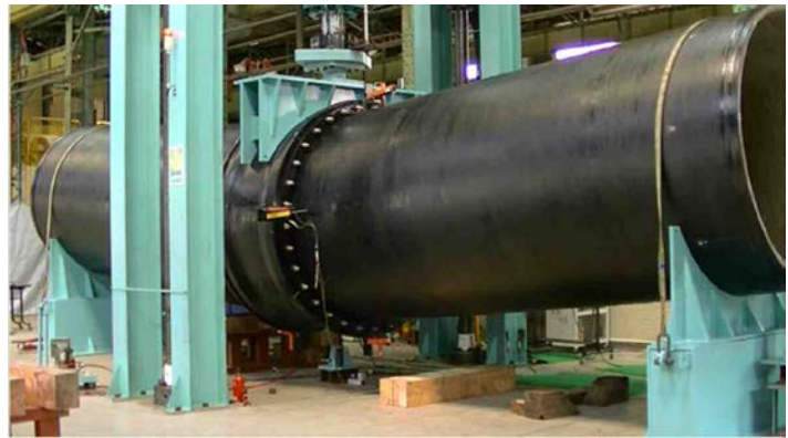
Fig. 3 – Full-scale tests of the joint performance of: (a) 60-inch diameter ERDIP performed in 2014 (left), (b) 72-inch S Type collar joint performed in September 2015 (right).
