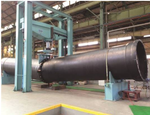
Fig. 3 – Full-scale tests of the joint performance of: (a) 60-inch diameter ERDIP performed in 2014 (left), (b) 72-inch S Type collar joint performed in September 2015 (right).
