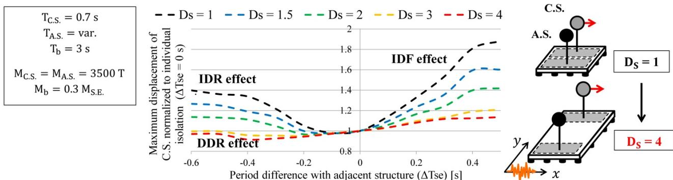
Fig. 9 - Structure-structure interaction as a function of system dispersion.
