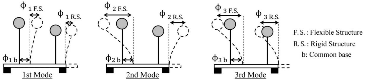
Fig. 4 - Two-structure base-isolated system modal forms in plane motion.
