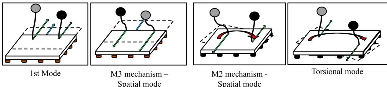
Fig. 8 - Two-structure base-isolated system modal forms in spatial motion.
