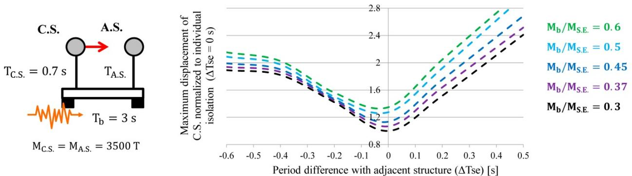
Fig. 7 - Influence of  $M_b/M_{S,E}$  ratio on structure-structure interaction.
