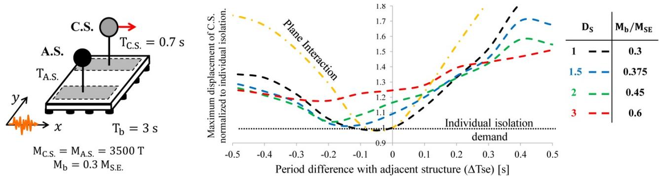
Fig. 10 – Structure–structure interaction as a function of system dispersion with variation of  $M_b$ .
