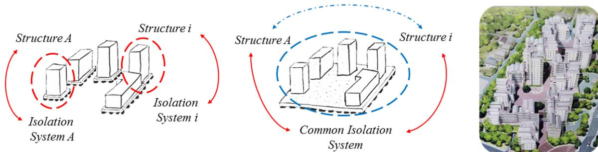
Fig. 1 – Multiple building – common base interaction schematized (left). Kamikuzawa Condominiums [4] (right).
