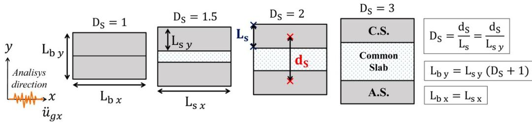
Fig. 3 - MB-BIs with different dispersion values measured on principal axis-x.
