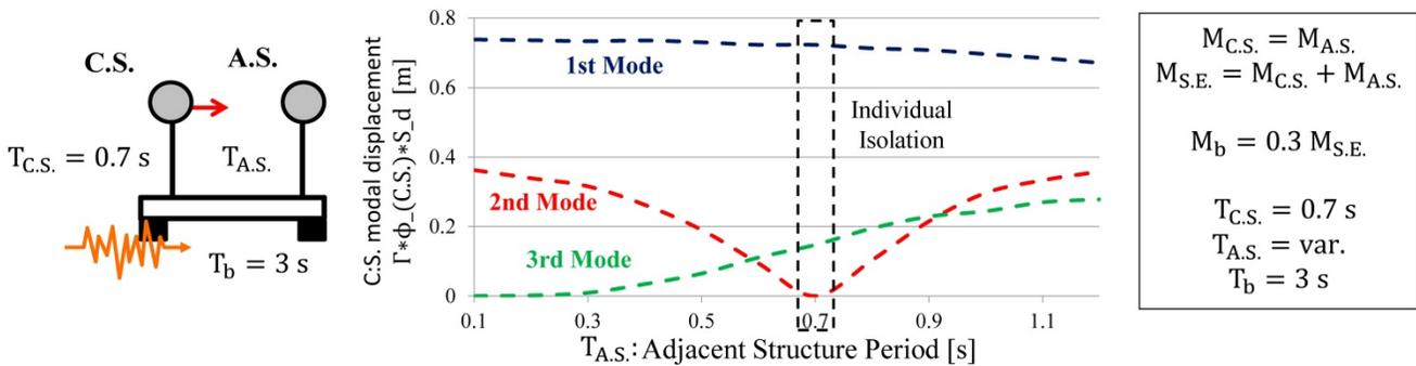
Fig. 5 - Modal displacement of C.S. as a function of A.S. period.
