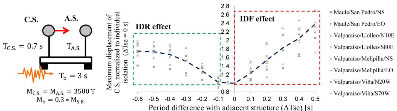
Fig. 6 - Displacement of C.S. as a function of A.S. period, normalized to individual isolation.
