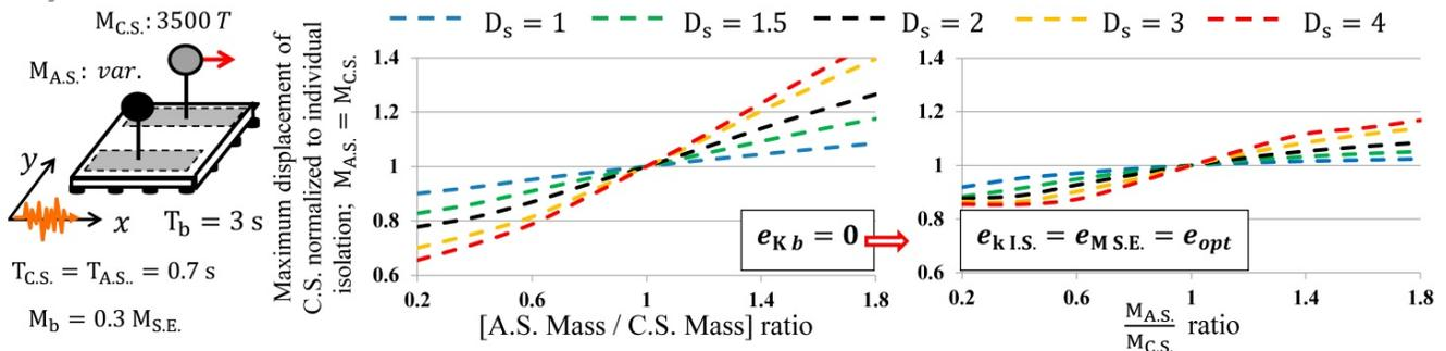
Fig. 12 - Structure-structure interaction caused by mass difference between structures.
