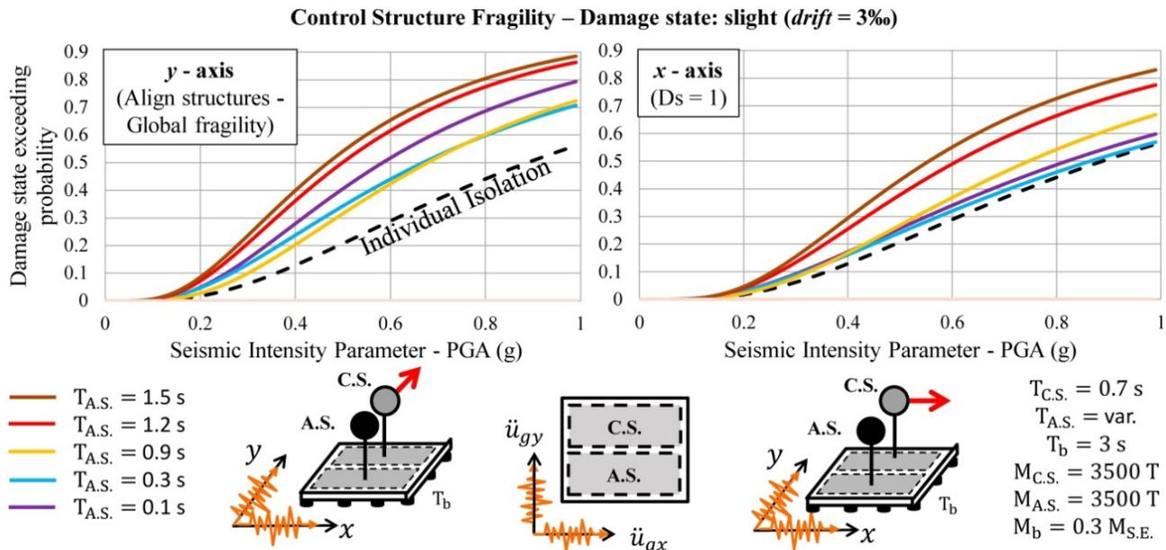
Fig. 11 - Control Structure fragility as a function of the Adjacent Structure period.
