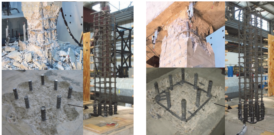
Fig.9. Two new cantilever specimens from RC-2. Application of short mechanical splice (left) and long mechanical splice (right).
