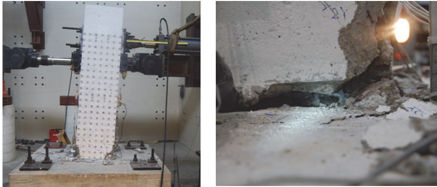
Fig.10. RC-2R-SMS at finishing of the test (left), new longitudinal bar broken and lifting at base (right)
