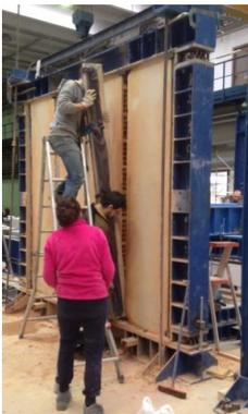
(d) insertion of the vertical joints [22]
