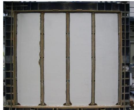
(f) downgraded infill before testing [22]
