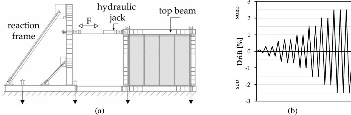
Fig. 10. Set-up (a) and loading protocol (b) for the in-plane test.
