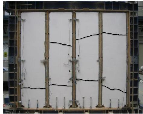
(b) crack pattern in the infill sub-panels at the end of the test
