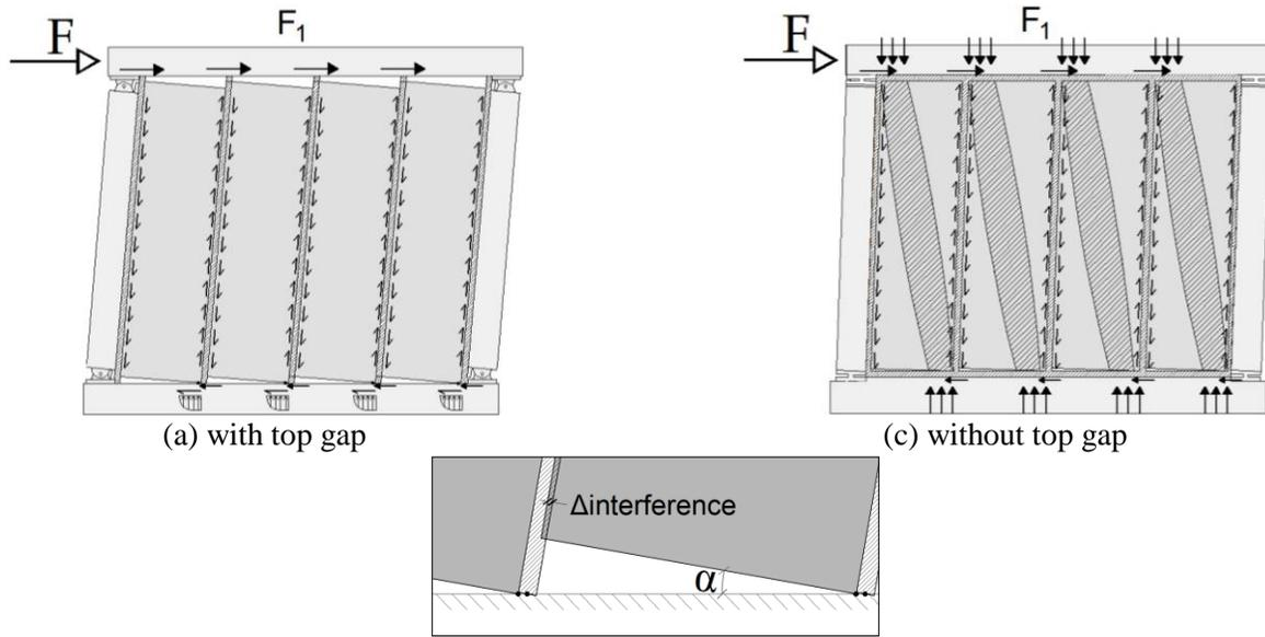
(c) ideal uplifting of the sub-panel and interference with the planks during the in-plane mechanism [22]
