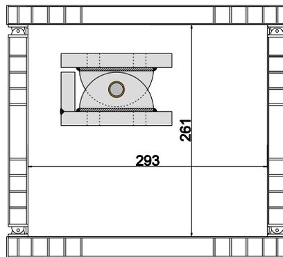
Fig. 7. Steel frame adopted in the tests with detail of the mechanical hinge at the column ends.
