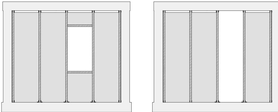
Fig. 3. Introduction of openings in the infill retrofitted with vertical elements.
