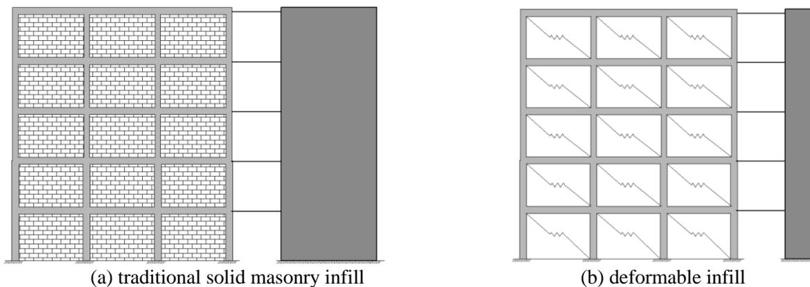
Fig. 2. Reduction of the additional bracing system size and stiffness for the retrofit of existing RC building, allowed by the downgrade of the infills.
