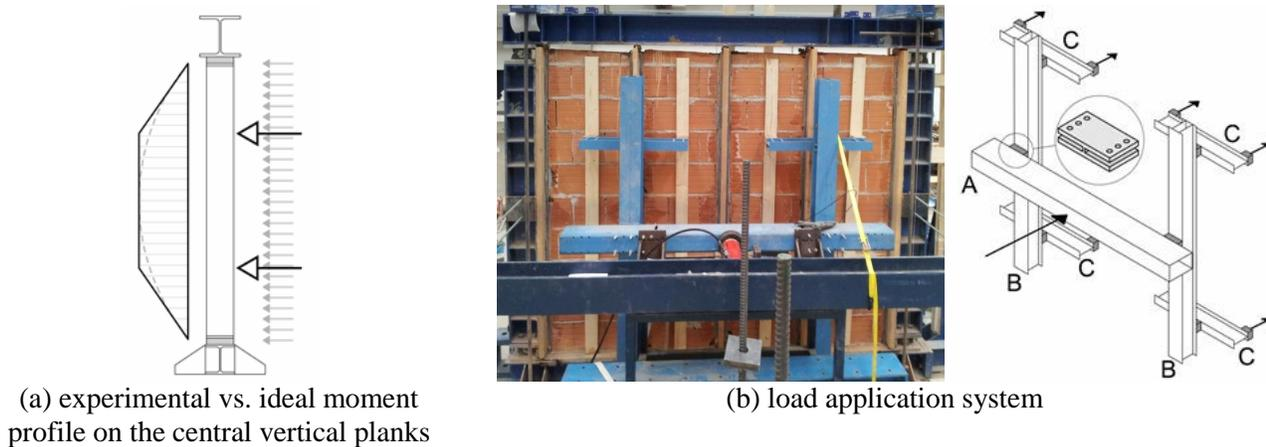
Fig. 12. Out-of-plane test set-up [22].
