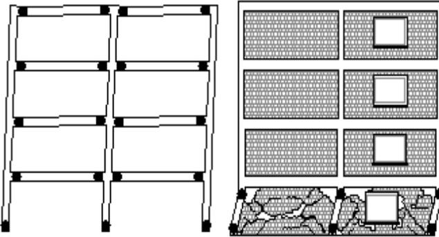
(a) modification of the frame collapse mechanism produced by the infill-frame interaction
