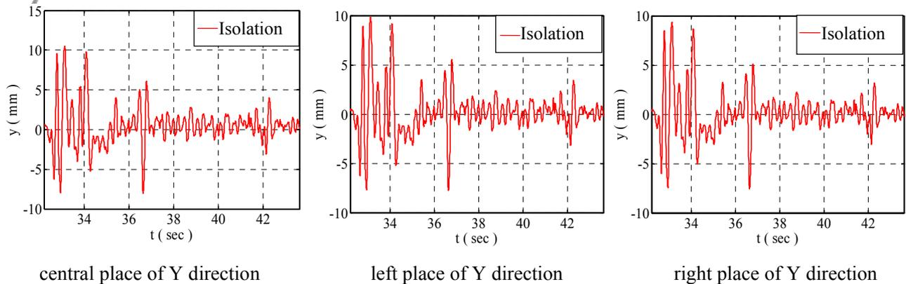
Fig.12—Displacement of isolation layer in inputting Y direction El Centro wave
