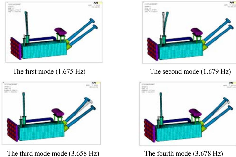
Fig.6 — Mode of converter transformer
