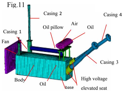
Fig.5 – Structure and FEM model of converter transformer
