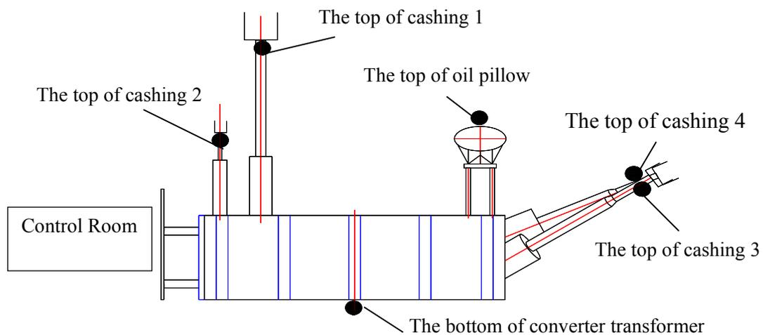
Fig.9 — layout of measuring points
