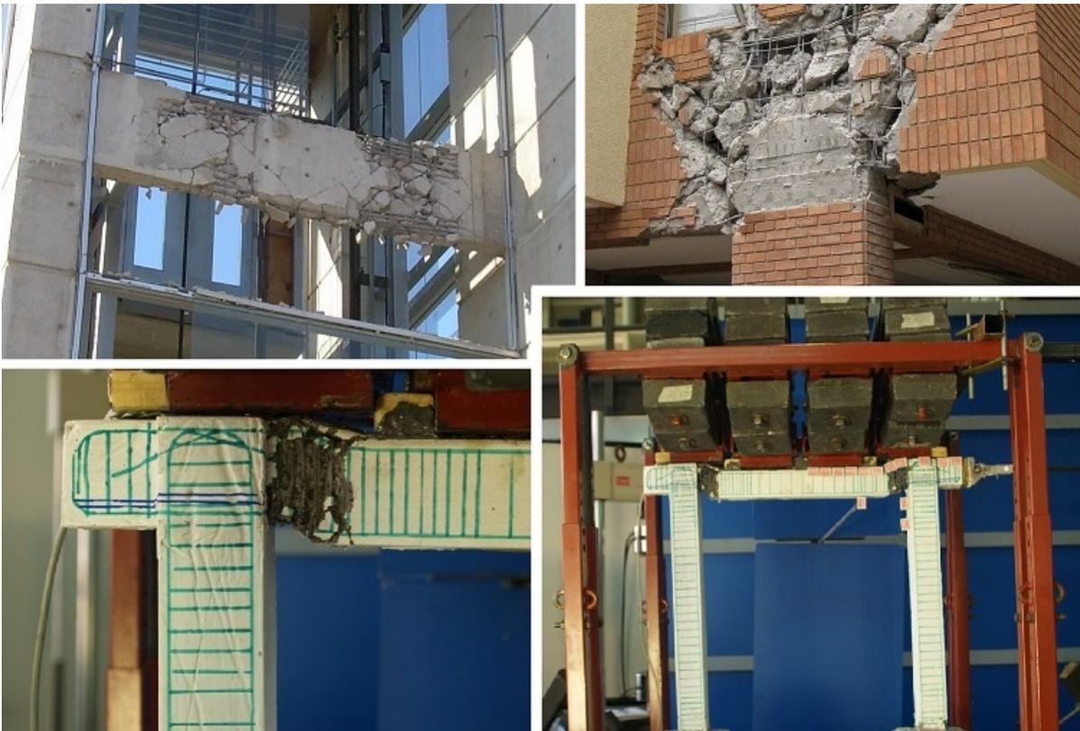
Fig. 1 - Damage concentration in real structures and scale models
