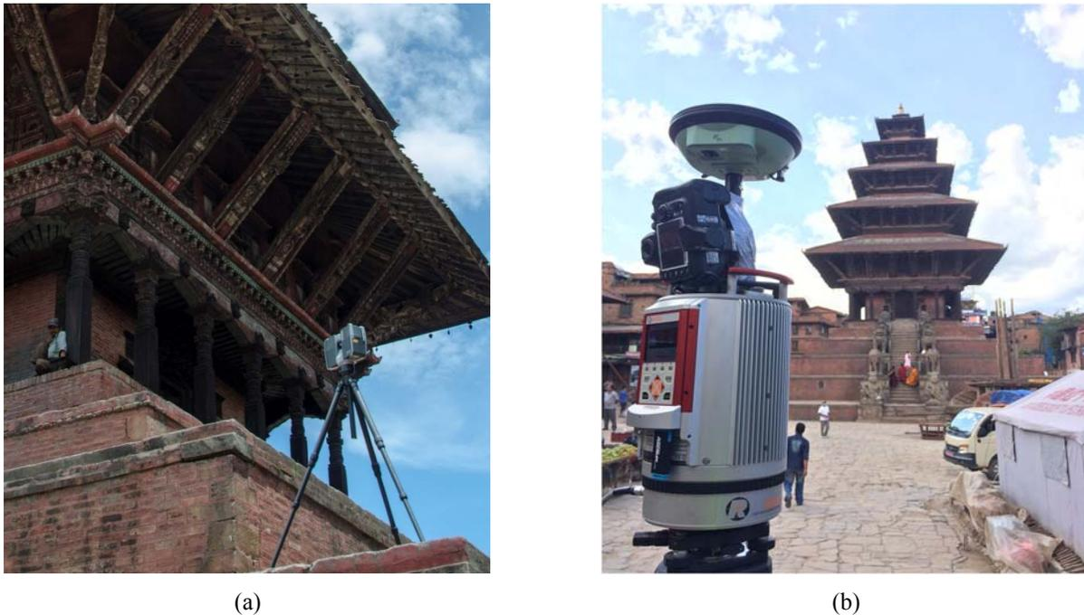
Fig. 3 – Lidar scanning at Bhaktapur’s Nyatapola Temple: (a) Faro Focus<sup>3D</sup> X 130 and (b) Riegl VZ-400 laser scanners.
