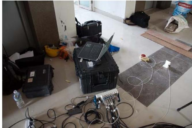
Fig. 5 – Example instrumentation implemented in the field: portable data acquisition, accelerometers, and field laptop.
