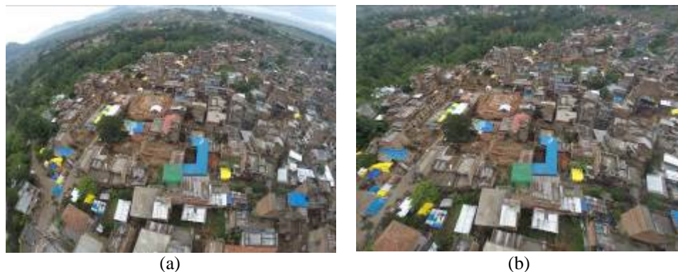
Fig. 6 - Example aerial image obtained from GoPro Hero 3+: (a) distorted image before correction and (b) after correction.
