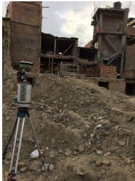
Fig. 9 - Riegl vz400 laser scanner with Leica GNSS GS14 on top.
