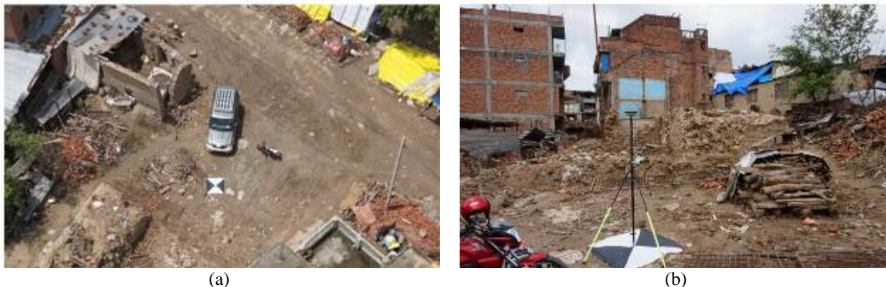
Fig. 3 - Demonstration of surveying technique: (a) an aerial target established in the study area, (b) GNSS rover station on an aerial target.
