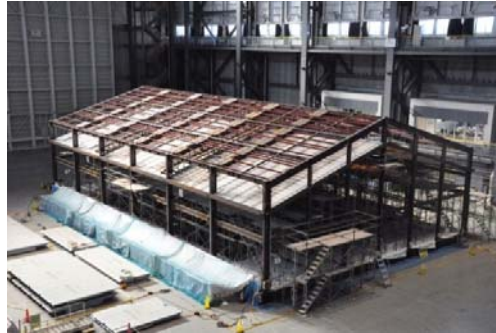
Photo 2 Full-scale Gymnasium Specimen
