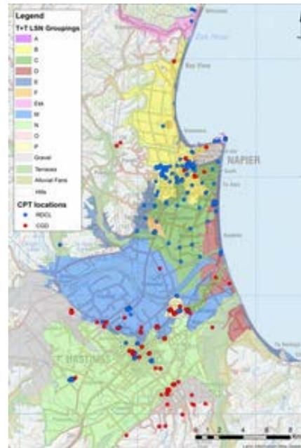
d) Liquefaction Zones: (Note: dots are CPT locations)
