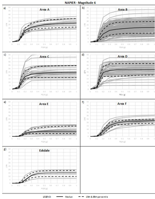
Figure 2 LSN vs PGA curves Mag 6 earthquake
