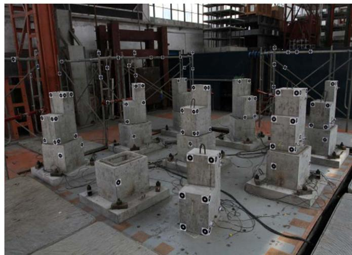
Fig. 9 – Damage state of models after 3-D shake test
