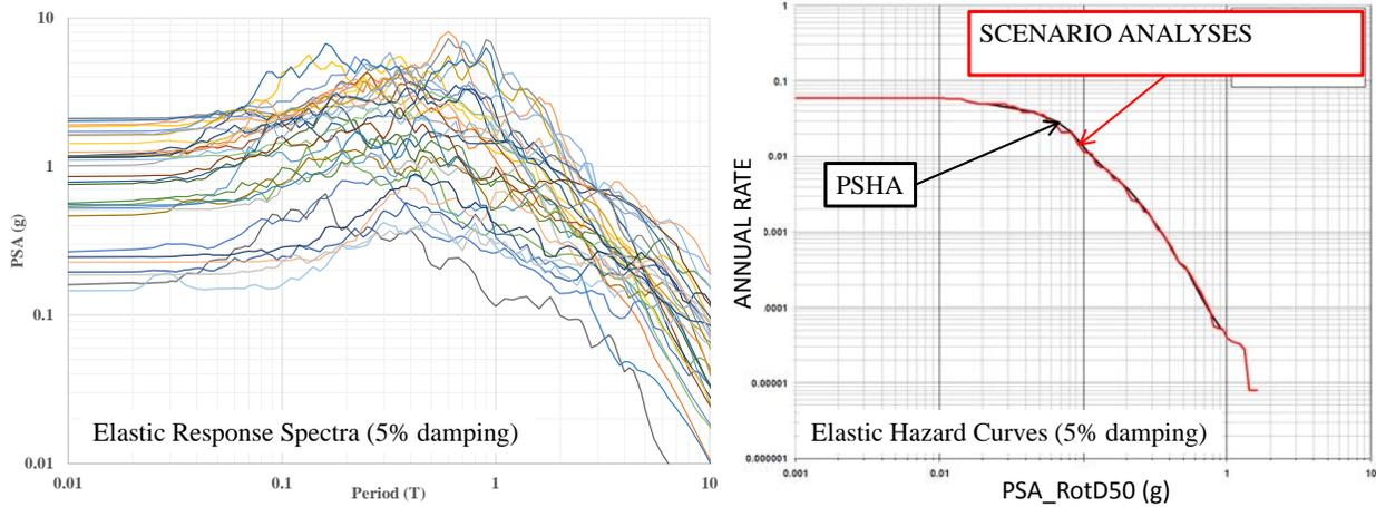
Fig. 6 Representative Elastic Response Spectra and Elastic Hazard Curves of Scenario Ground Motions
