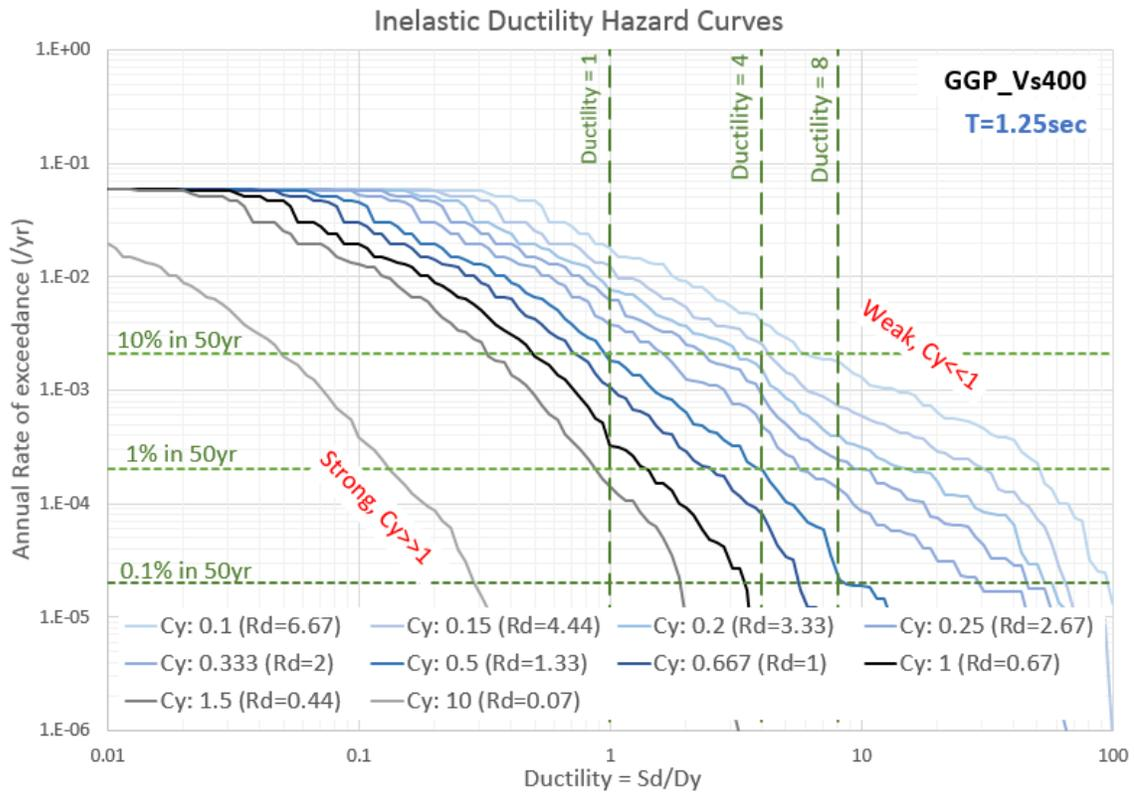
Fig. 8 Inelastic Ductility-Hazard Curves for GGP Site, T=1.25s
