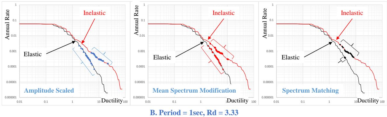
Fig. 10. Interpolation of Ground-Motion Response on Hazard Curves
