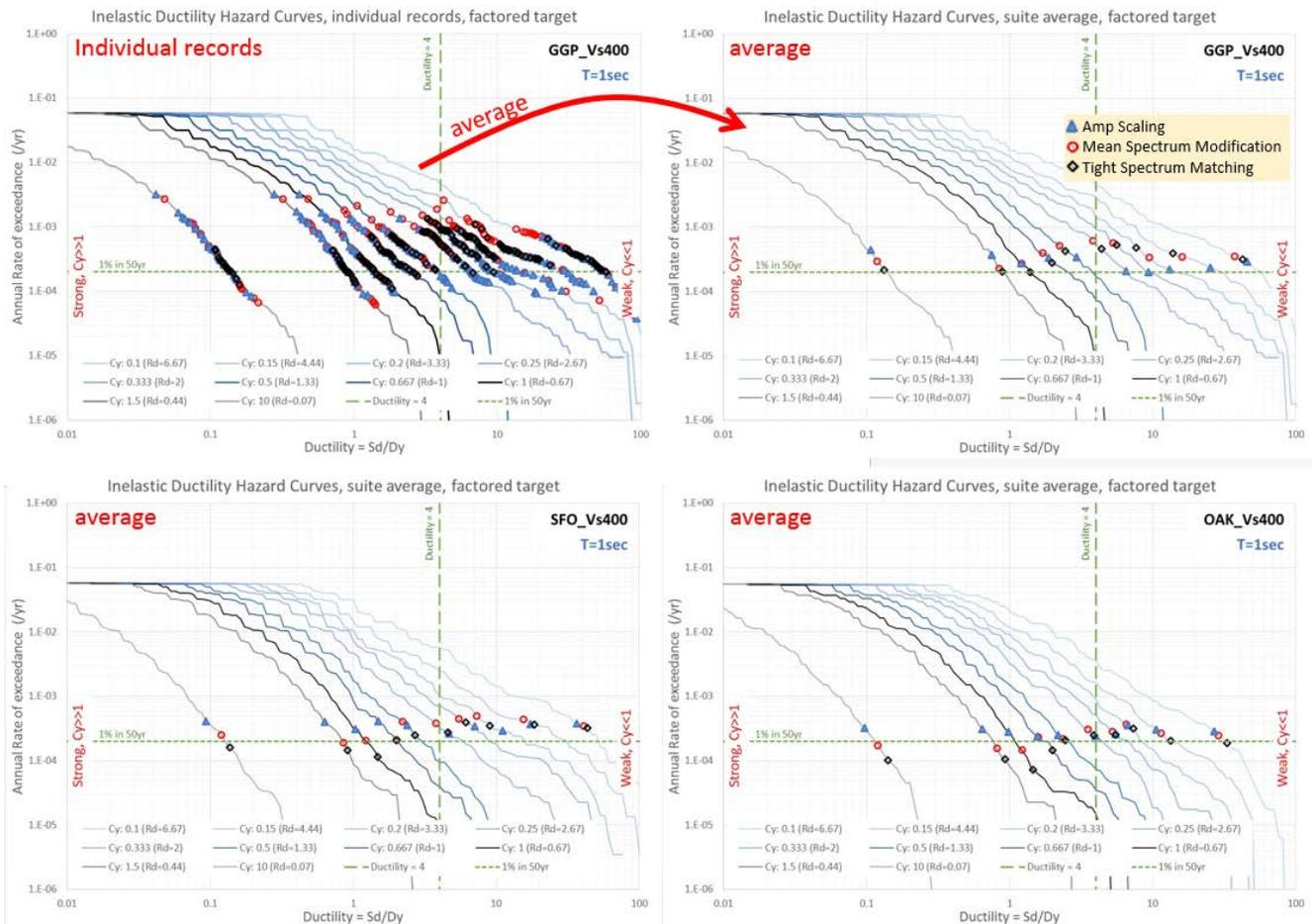
Fig. 11. Ground-Motion Response & Inelastic Ductility Hazard Curves (Blue Triangle=Amplitude scaling, Red Circle=Mean Spectrum Modification, black Diamond=Tight Spectrum Match)
