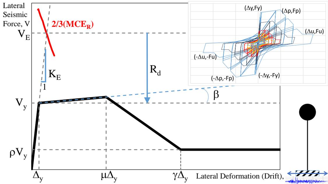
Fig. 5 Simplified SDOF Nonlinear Inelastic Structural Model in OpenSees
