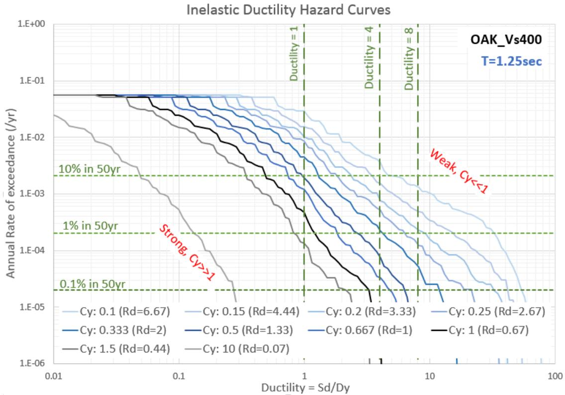
Fig. 9 Inelastic Ductility-Hazard Curves for OAK Site,  $T=1.25s$
