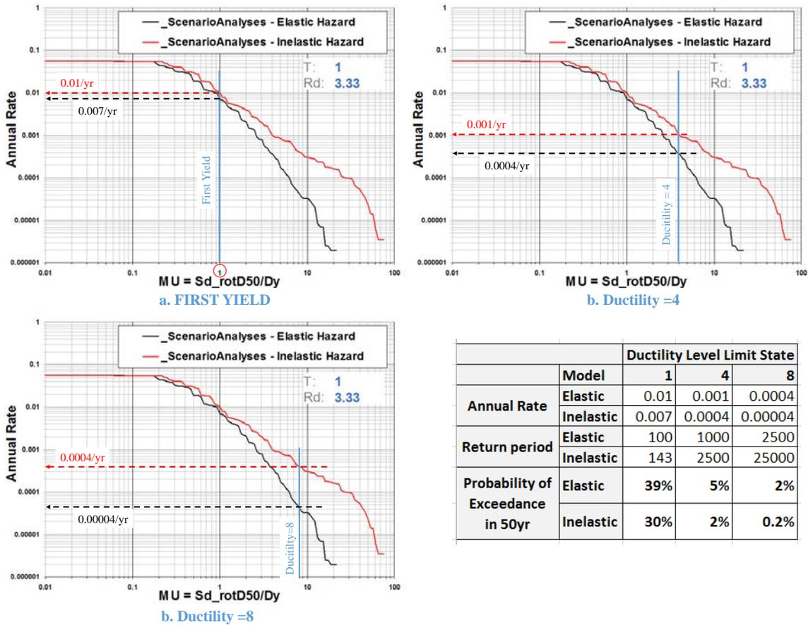
Fig 7. Comparison of Elastic Inelastic Hazard Curves for Typical Site, T=1, Rd=3.33
