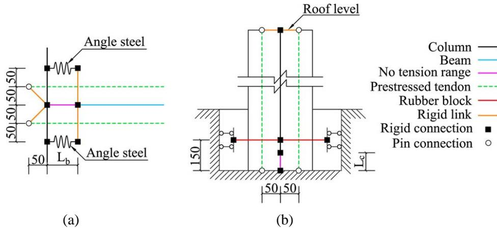
Fig. 9 – Computational models: (a) beam-column joints, and (b) column-base joints
