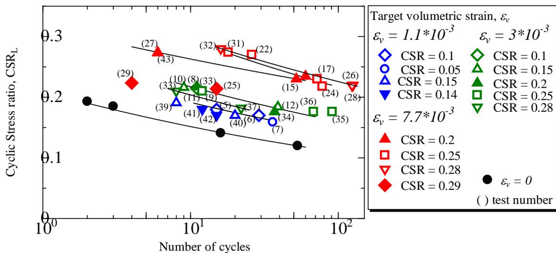
Fig. 2 – Relationship between cyclic stress ratio and number of cycles
