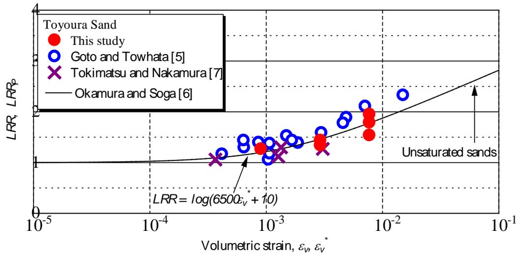
Fig. 4 – Relationship between rates of increase in  $LRR$  and volumetric strain: comparison of pre-shaking effects with unsaturated and membrane penetration effects
