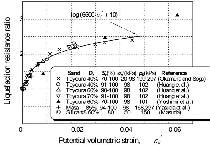
Fig. 3– Relationship between potential volumetric strain and liquefaction resistance ratio of partially saturated sand (after Okamura and Soga [6])
