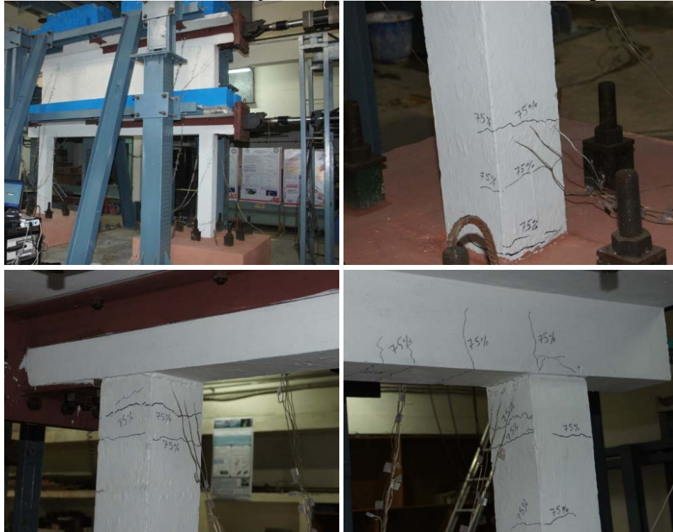
Fig. 9 – Test frame with loading condition and various damage on ground column in 75% Electro
