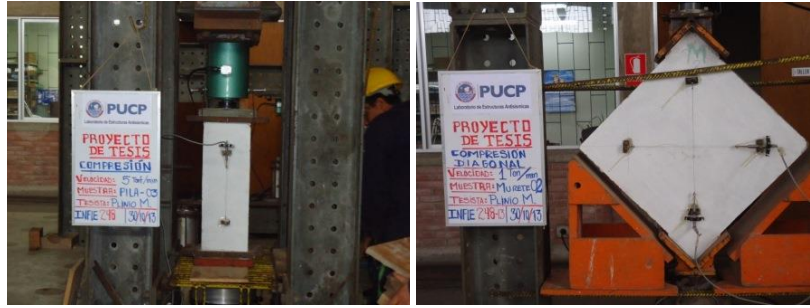
Fig. 4 – Masonry tests on axial compression (left) and diagonal compression (right).
