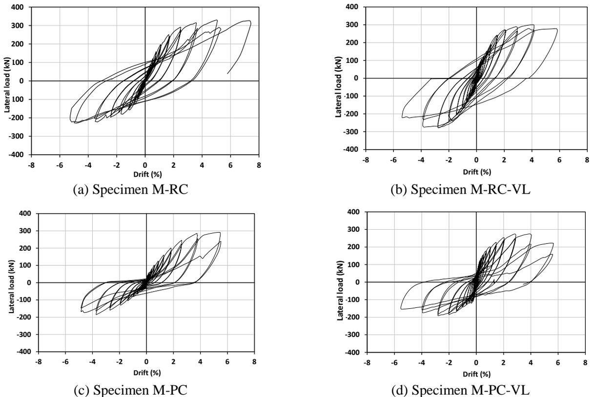
Fig.3 – Lateral load-drift relation of specimens.
