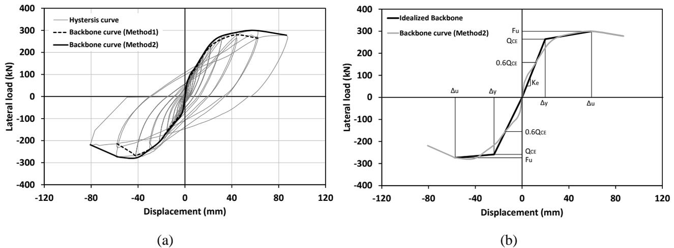
Fig.4 – (a) Backbone curves of specimen M-RC-VL; (b) Idealized of backbone curve (Method2) of specimen M-RC-VL.
