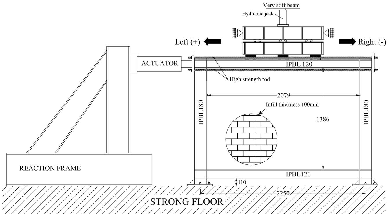
Fig. 1 – schematic view of test setup, dimension in mm.
