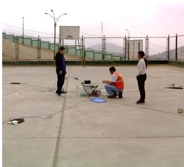
Photo 2. Microtremor Array Test in the Ventanilla district
