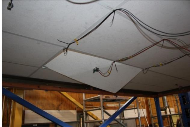
Figure 16 - Panel dislodgment in the final sinusoidal test
