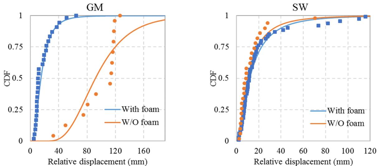
Figure 15 - Distribution of ceiling peak relative displacement in ground motion (GM) and sinusoidal (SW) tests, with and without isolation foam
