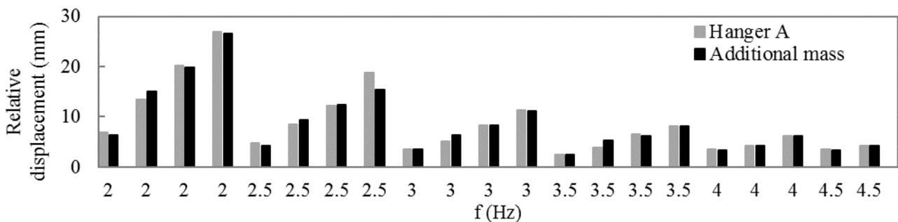
Figure 7 - Peak relative displacement in sinusoidal tests, hanger layout "A" with and w/o added mass
