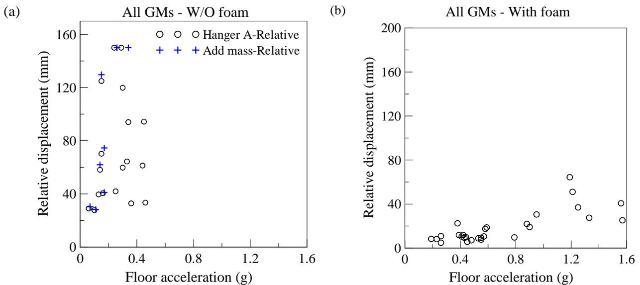
Figure 5 - Ceiling peak displacement in ground motion tests
