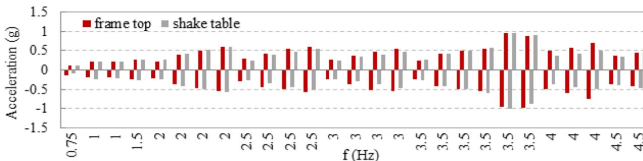
Figure 3 – Acceleration recorded on shake table and acceleration response on frame top
