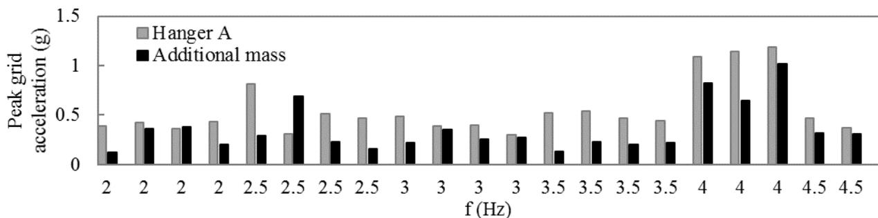
Figure 8 - Peak grid acceleration at ceiling centre, hanger layout A, with and w/o added mass
