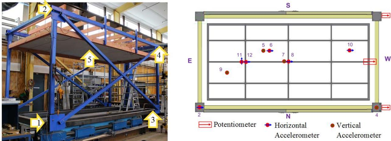
Figure 2 – Instruments on test frame and test specimen
