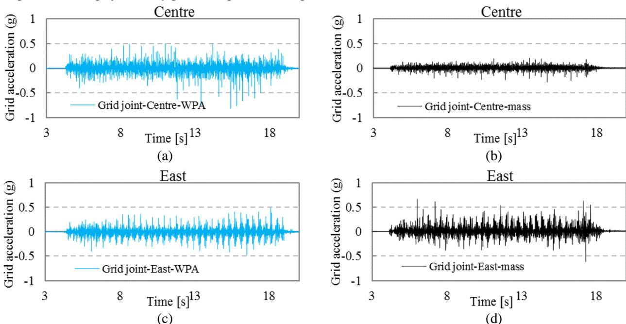
Figure 10 - Horizontal acceleration time histories on ceiling grid in sinusoidal tests (a & c) with and, (b & d) w/o added mass
