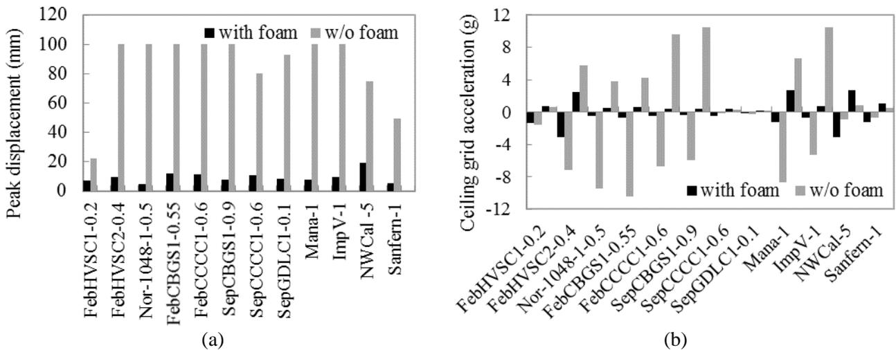
Figure 13 - (a) Peak ceiling displacement; and (b) acceleration on central grid joint w/ & w/o foam
