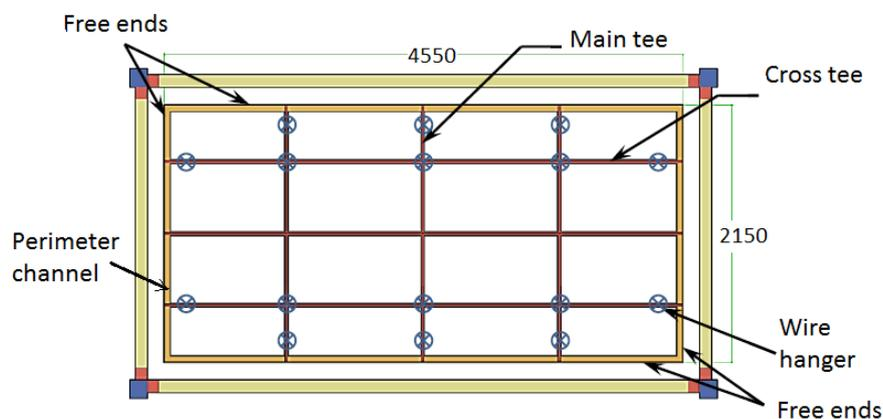
Figure 1 – Plan view of fully-floating ceiling specimen
