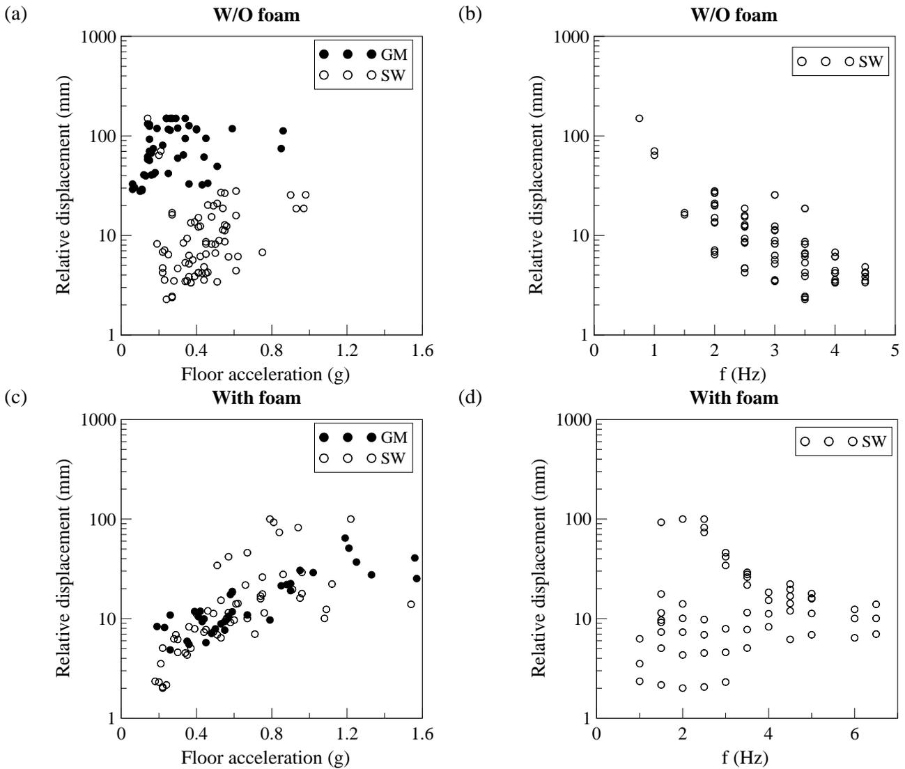
Figure 12 - Peak ceiling relative displacement in sinusoidal (SW) and ground motion (GM) tests w/ & w/o foam
