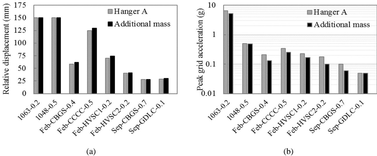
Figure 6 - (a) Peak ceiling relative displacement, and (b) grid acceleration in ground motion tests
