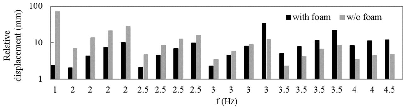
Figure 14 - Peak ceiling displacement with and without foam isolation in sinusoidal tests.
