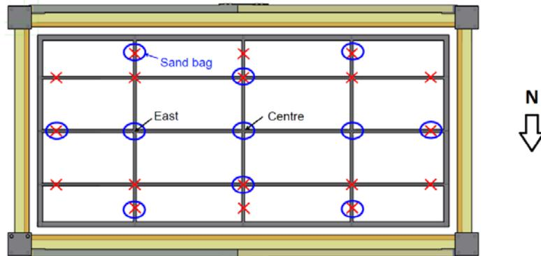
Figure 9 - Plan view of specimen with hanger layout A, position of sand bags and centre and east grid joints
