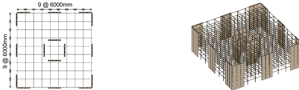
Fig. 2.1 – Sample layout with twenty-four walls
