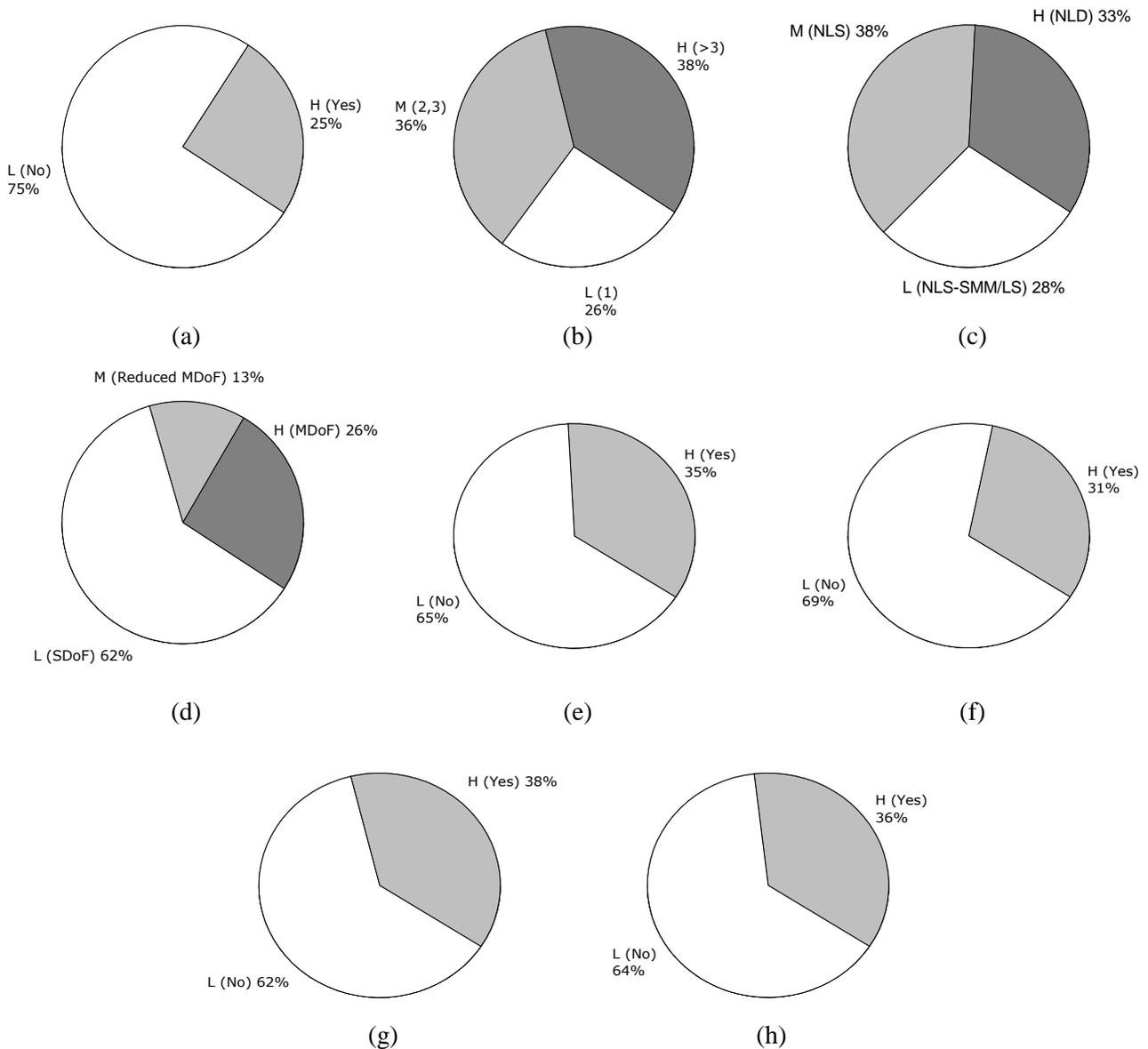
Fig. 4 – Percentage of fragility curves regarding capacity-related features: non-structural components (a), classes of building height (b), analysis type (c), model type (d), shear failure of reinforced concrete elements (e), out-of-plane mechanism in masonry buildings (f), horizontal diaphragms (g) and geometric irregularities (h)
