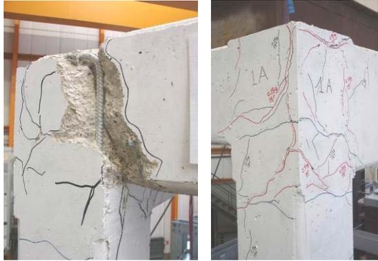
Fig. 2 – Damage in 2<sup>nd</sup> floor joints after the test  $PGA=0.15g$  on original building
