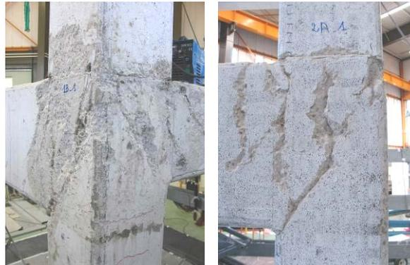
Fig. 4 – Damage at 1<sup>st</sup> floor joints after tests on the PTMS-strengthened building
