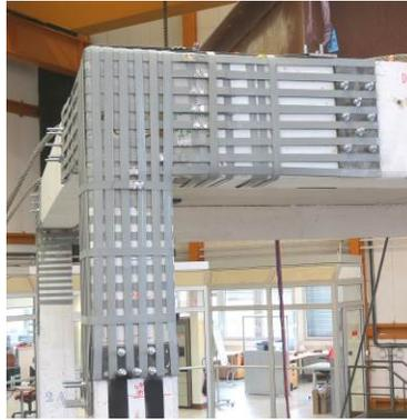
Fig. 3 – View of a typical PTMS-strengthened 2<sup>nd</sup> floor joint
