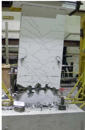
Fig. 2 – Condition of Wall W2-NR prior to failure (Abdulridha [1])
