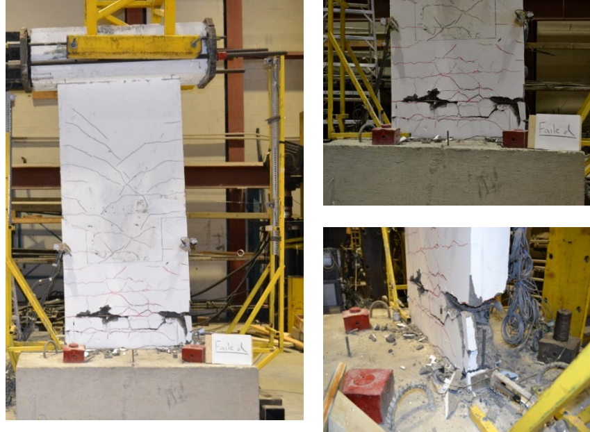
Fig. 9 – Damage state of Wall RW2-NR at the end of testing
