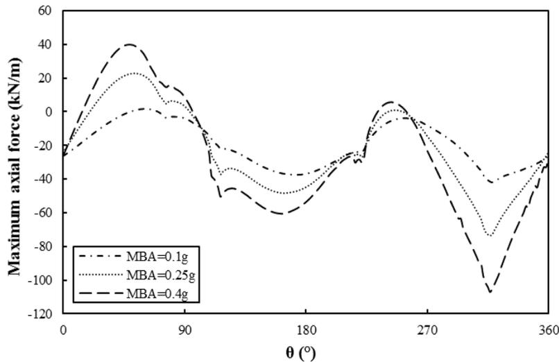
Fig. 7 – Variation of axial force in the tunnel lining at different base accelerations
