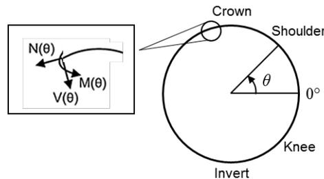
Fig. 2 – Sign convention used to measure lining forces
