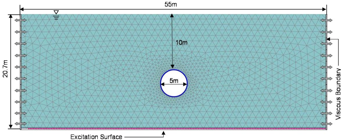
Fig. 1 – FE model of tunnel-soil system
