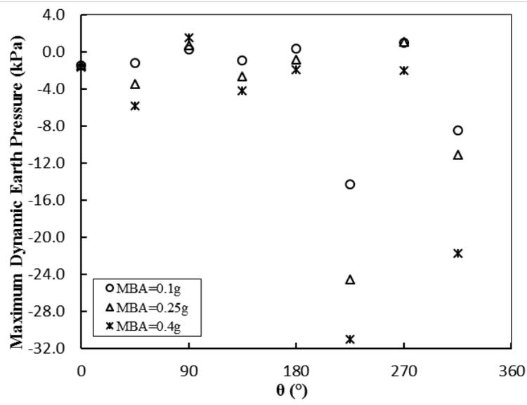
Fig. 5 – Maximum dynamic earth pressures around the tunnel lining at different base accelerations
