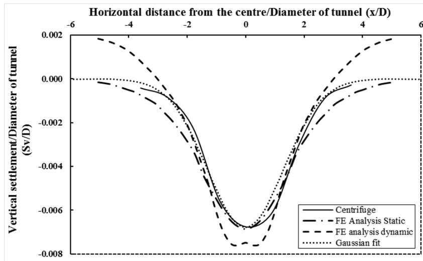
Fig. 3 – Comparison of surface settlement profile of a single circular tunnel
