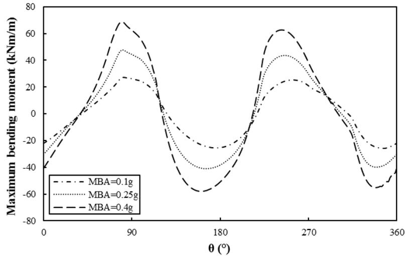
Fig. 8 – Variation of bending moment in the tunnel lining at different base accelerations
