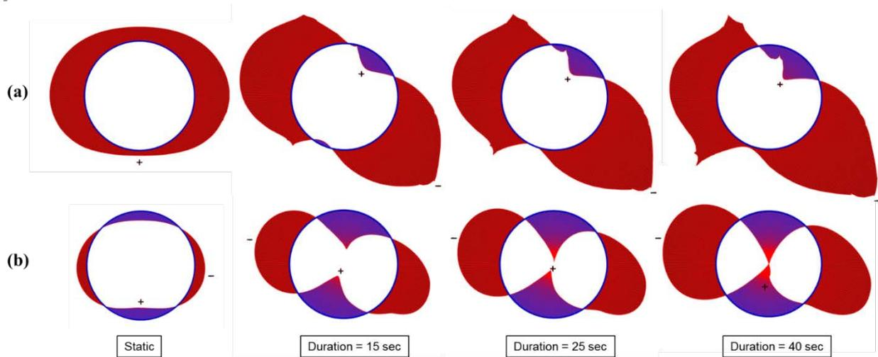
Fig. 9 –Variation in tunnel lining forces under static and seismic loading with duration: (a) axial forces, (b) bending moments
