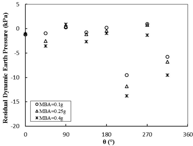
Fig. 6 – Residual dynamic earth pressures around the tunnel lining at different base acceleration
