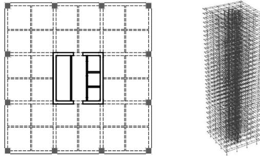
Fig.1 Layout of structures and 30-storey reference building model in Perform-3D
