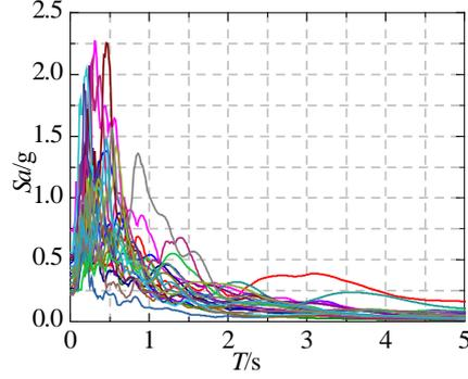
Fig.2 (Pseudo-) Acceleration response spectra of ground motions (5% damping)
