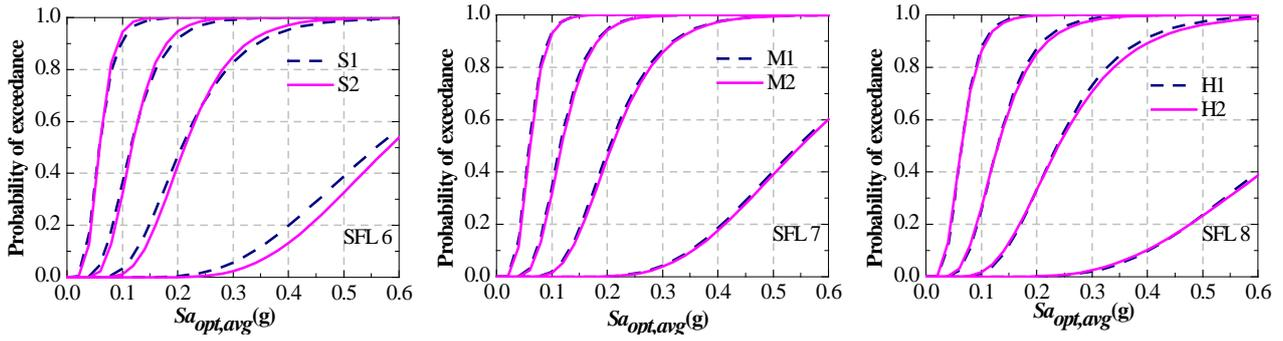
(a) Seismic fragility curves of reference structures with varying plan width (18m and 24m)
