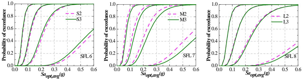
(b) Seismic fragility curves of reference structures with varying story ( 20 story and 30 story)
