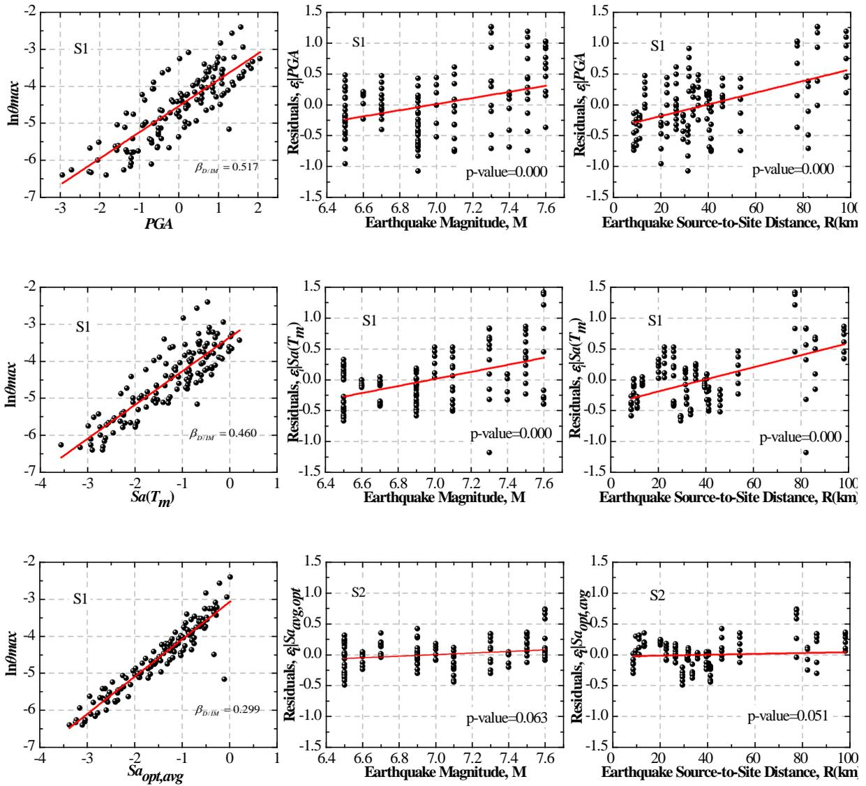
Fig.3 Efficiency and sufficiency property considering different IMs of the building S1
