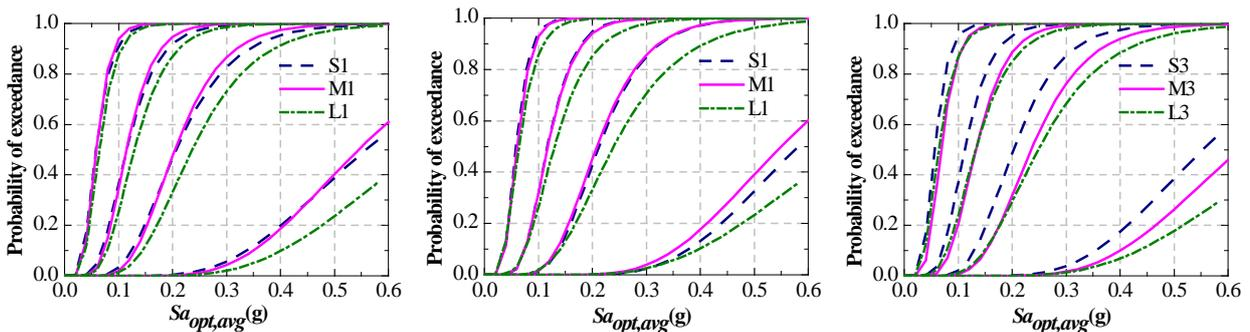
Fig.5 Seismic fragility curves of structures under different seismic fortification level
