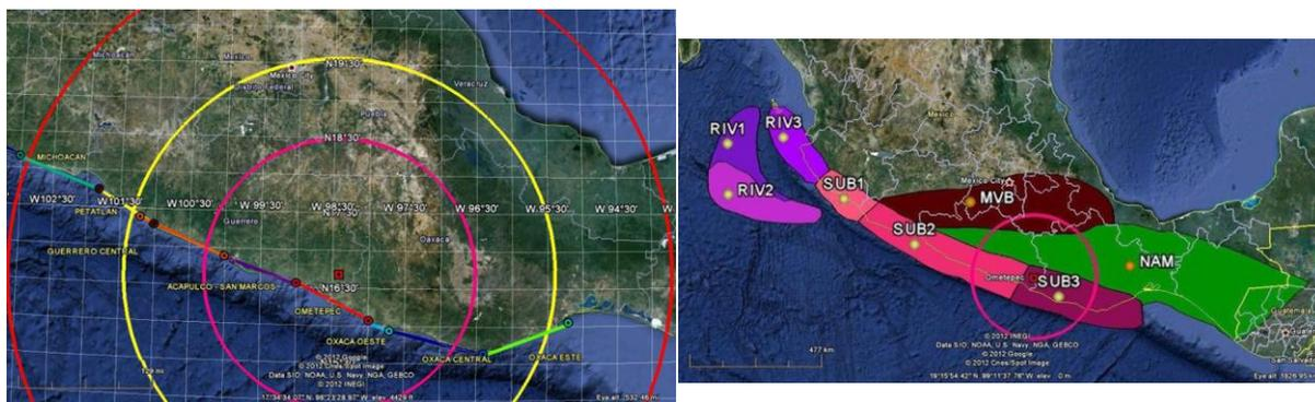
Fig. 1 - Seismic sources for Ometepec: Left, Fault types; Right, Area types.
