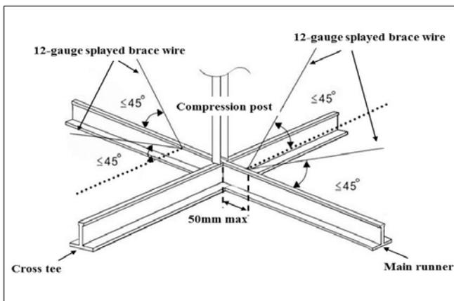
Fig. 1 – Details for the bracing assembly
