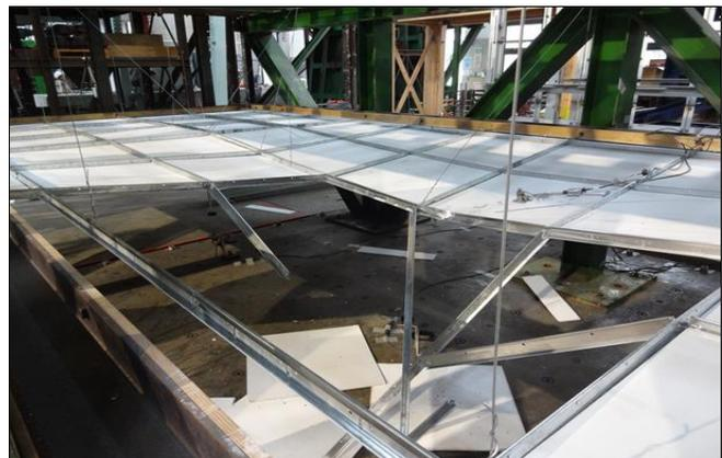
Fig. 14 – Collapse of the ceiling system
