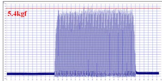
Fig. 21 – Tensile force of the splayed wire
