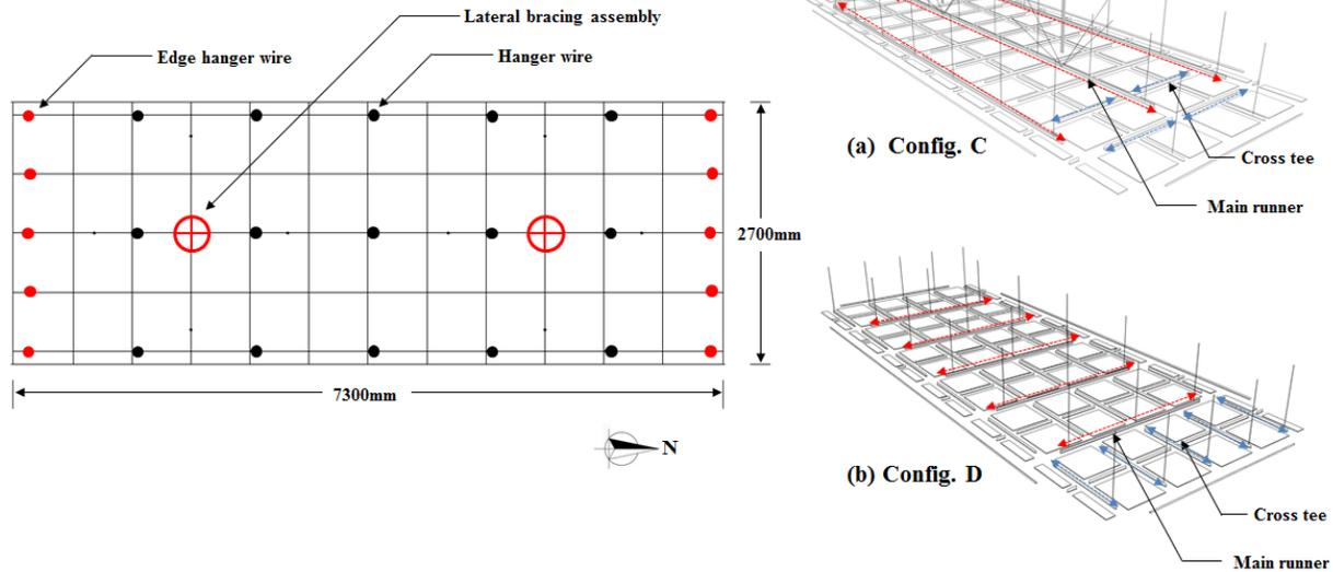
Fig. 10 – Overall view of the ceiling system in the second series of experiments
