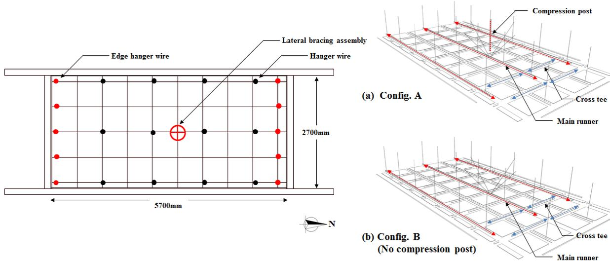
Fig. 5 – Overall view of the ceiling system in the first series of experiments
