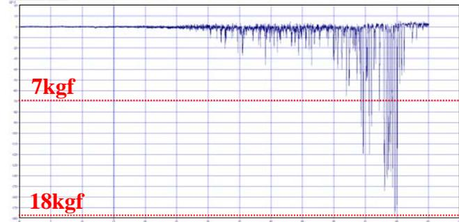
Fig. 23 – Tensile force of the splayed wire
