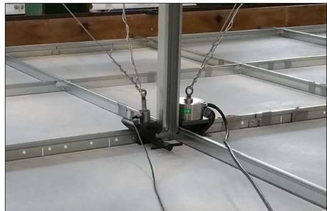
Fig. 9 – Installation of the load cell
