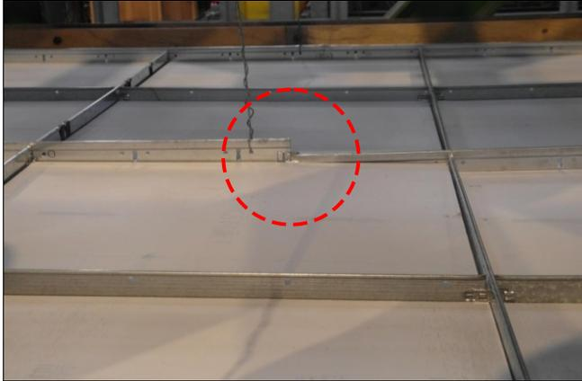
Fig. 11 – Detachment of the main runner joint
