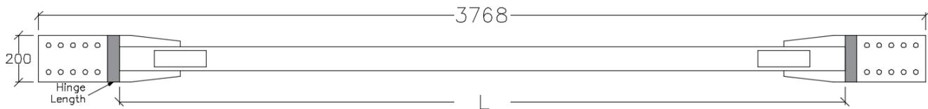
Figure 7 – Specimen diagram (units in mm)
