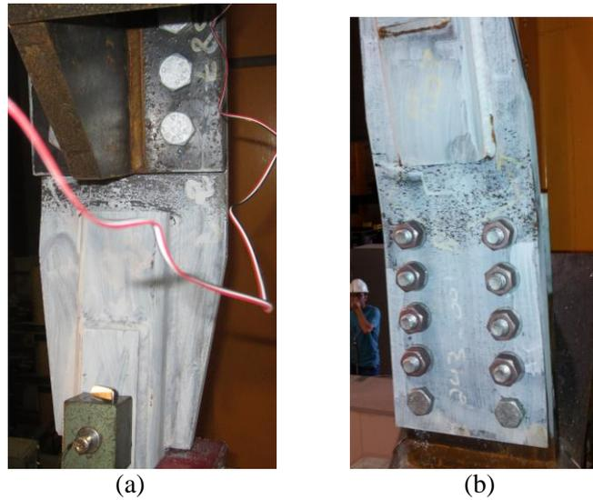
Fig. 10 – Rotation in the hinge plates under peak compressive displacement: (a) Top hinge plate (Specimen #1); (b) Bottom hinge plate (Specimen #2)
