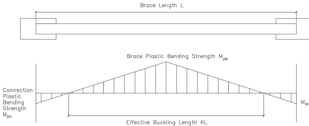
Fig. 12 – Determination of effective buckling length factor K
