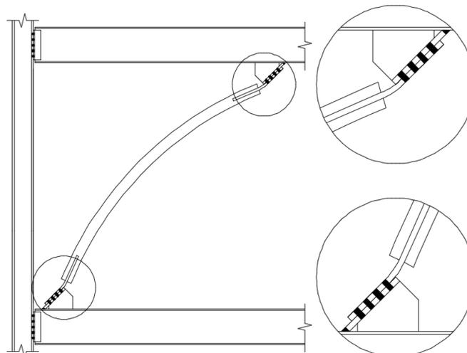
Fig. 3 – Connection rotation at brace ends
