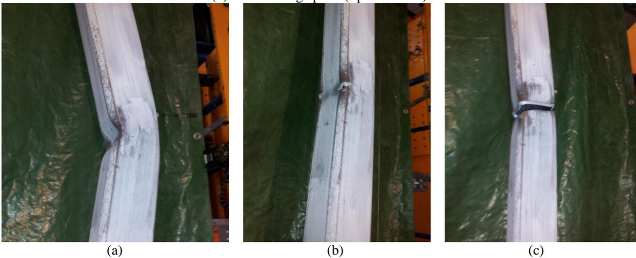
Fig. 11 – Brace failure progression (Specimen #2): (a) Significant local buckling; (b) Tensile tears form; (c) Complete fracture
