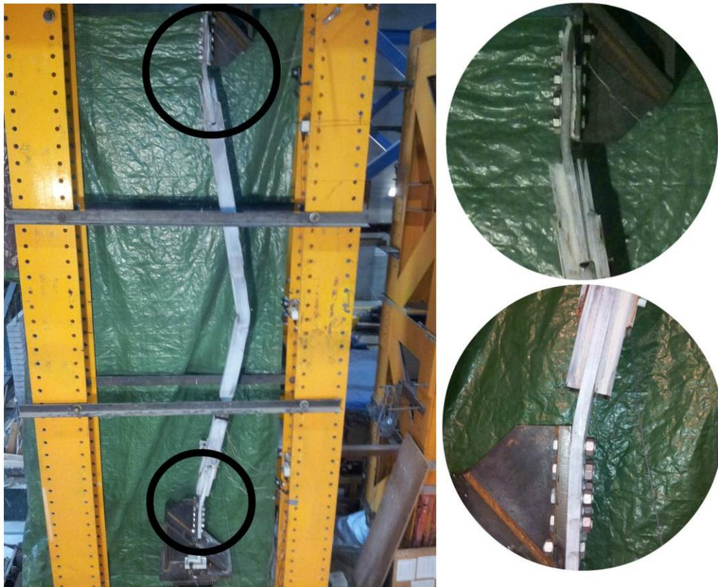
Fig. 9 – Rotation in the hinge plates under peak compressive displacement (Specimen #2)
