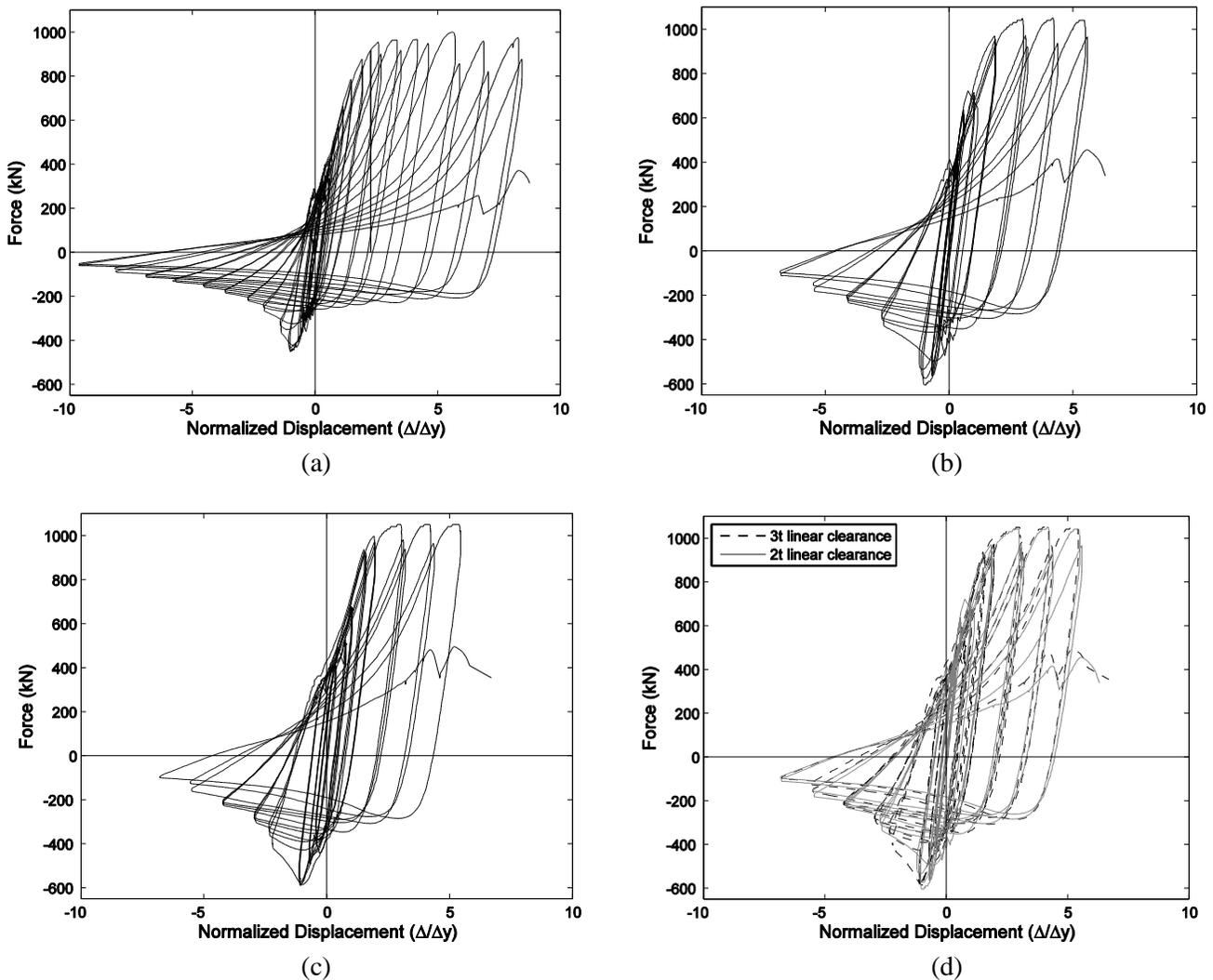
Fig. 8 – Cyclic force-deflection curves: (a) Test specimen 1; (b) Test specimen 2; (c) Test specimen 3; (d) Test specimens 2 (2t clearance) and 3 (3t clearance)
