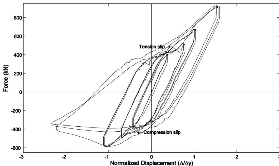
Fig.13 – Bolt slip at low displacements (Specimen #3)
