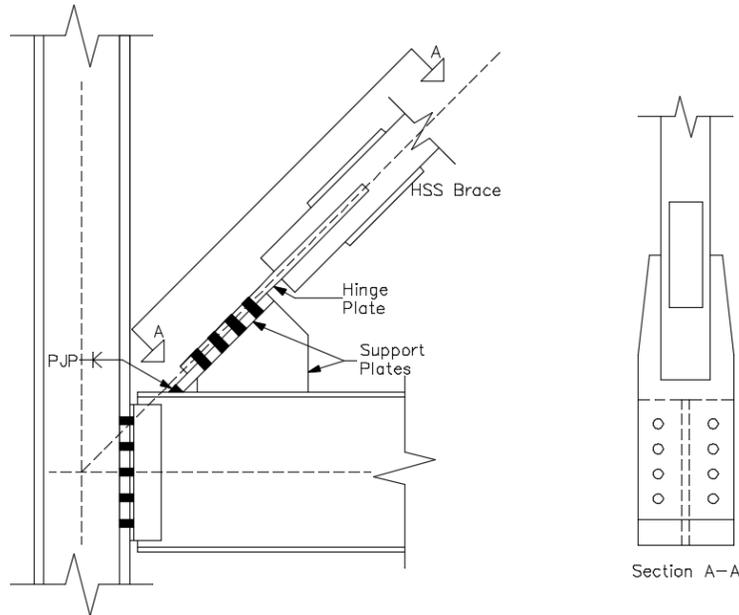
Fig. 2 – Proposed connection design
