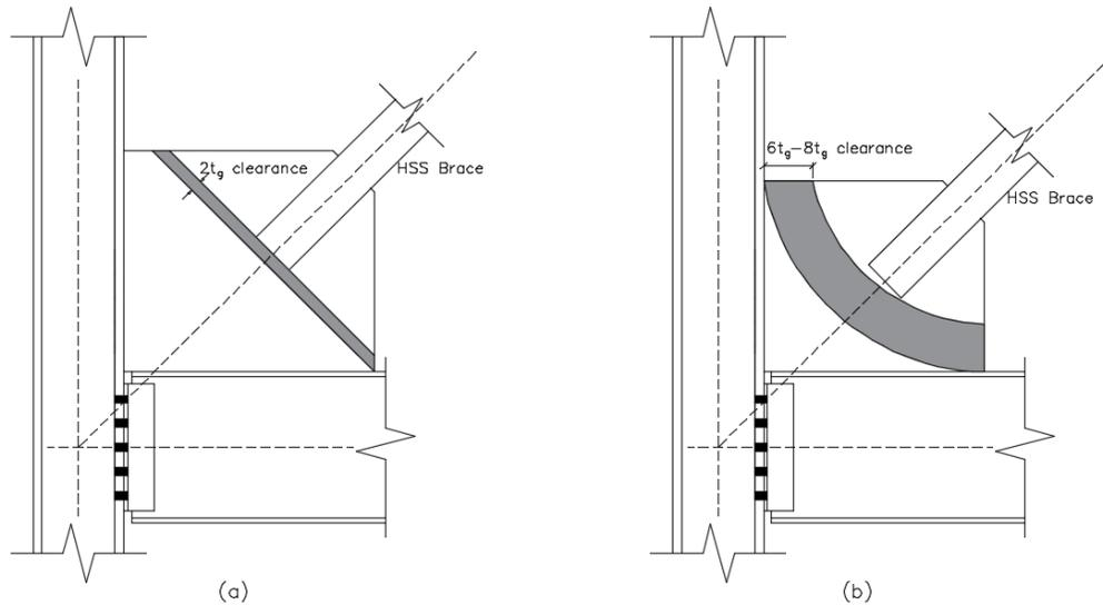
Fig. 1 – Typical CBF gusset plate designs: (a) Linear clearance rule; (b) Elliptical clearance rule
