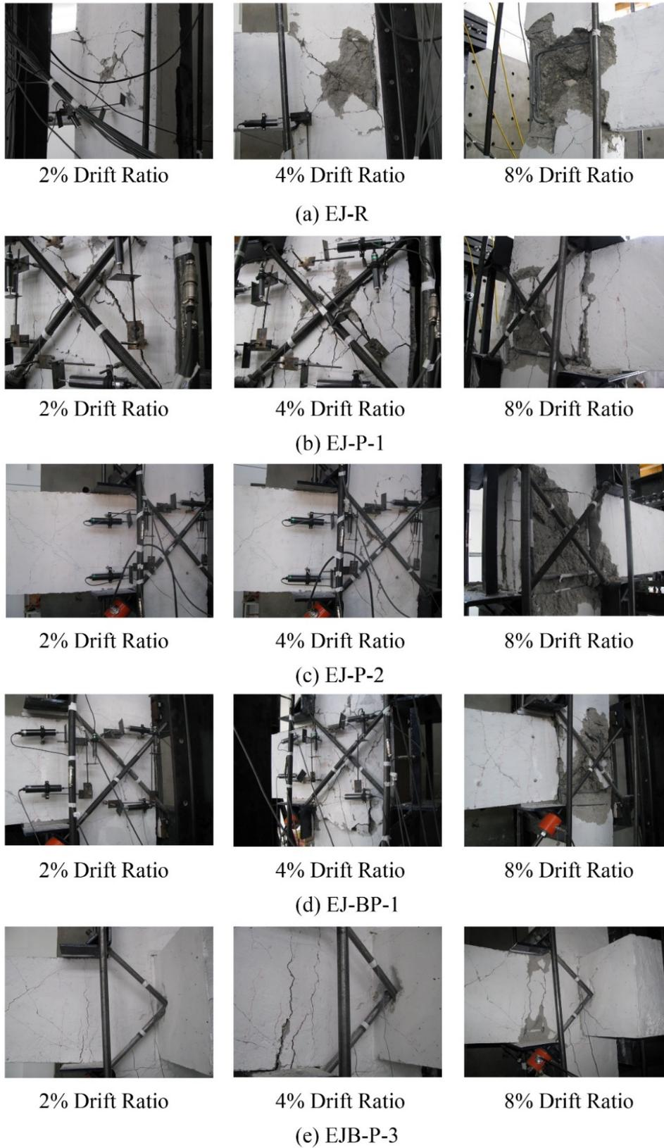
Fig. 4. Photographs of the damaged specimens at 2%, 4% and 8% drift ratios
