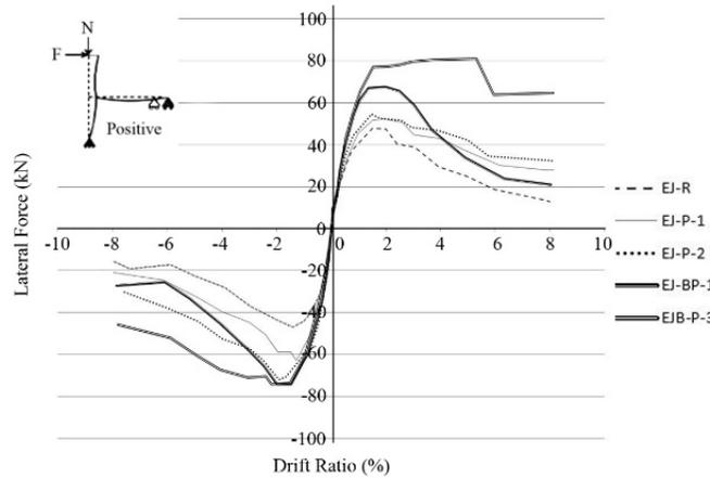
Fig. 6. Envelope curves of each tested specimen
