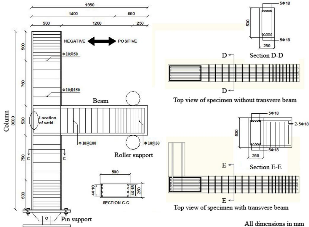
Fig. 1. Dimensions and reinforcement details
