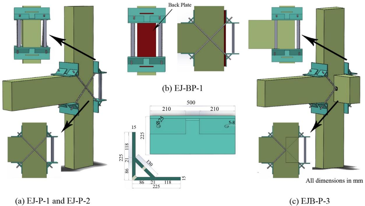
Fig. 3. Schematic representations of post-tension detail
