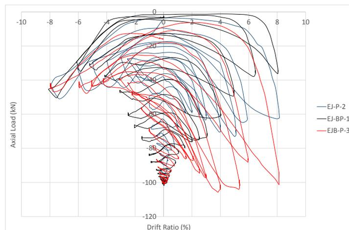
Fig. 7. Change in the axial force in the rods
