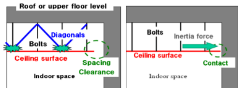
(a) with spacing and braces (b) w/o spacing or braces Fig.1 JPN style ceiling
