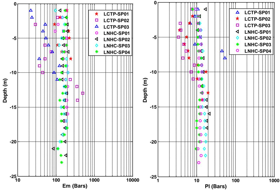
Fig. 2: Profile of Pressuremeter parameters at Algiers site
