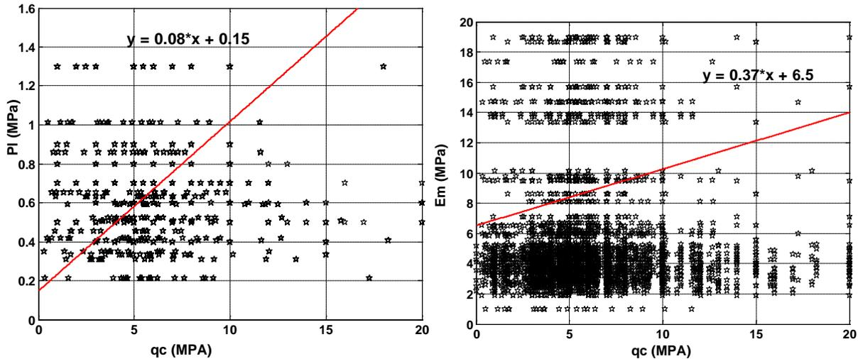
Figure 5. Relation between pressuremeter parameters and cone penetration resistance of sand and fitted relations
