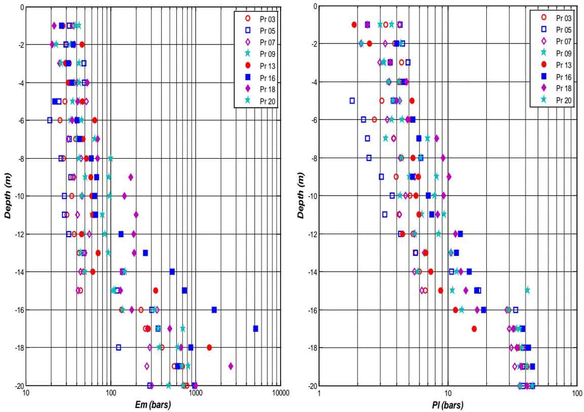
Fig. 1: Profile of Pressuremeter parameters at Mostaganem site
