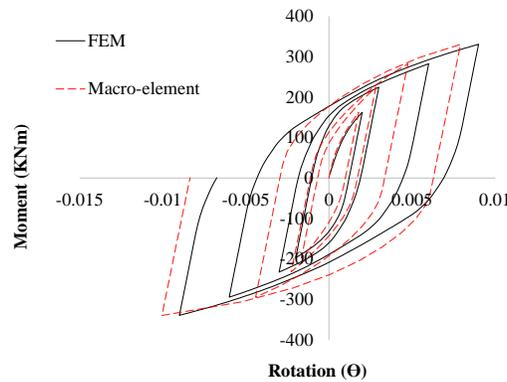
**Fig. 5. Quasi-static load for moment vs. rotation at the foundation**
