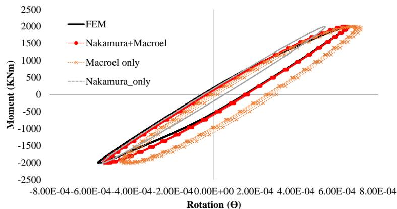
**Fig. 7. Hysteretic loop for simplified models and FEM model with cyclic moment load**
