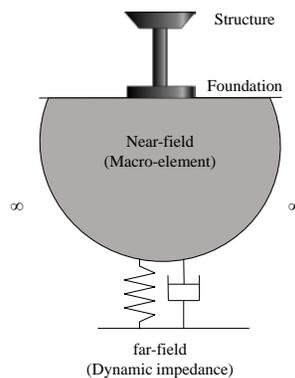
**Fig. 1. Schematic diagram of macro-element with far-field soil domain**
