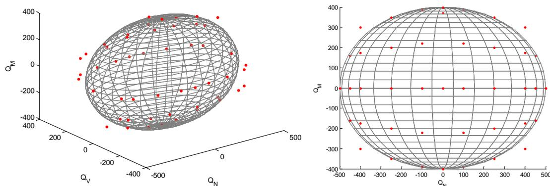
**Fig. 4. Bounding surface generated from FEM and macro-element**
