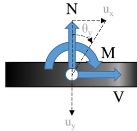
**Fig. 2. Generalized force and displacement diagram for shallow foundation in macro-element**
