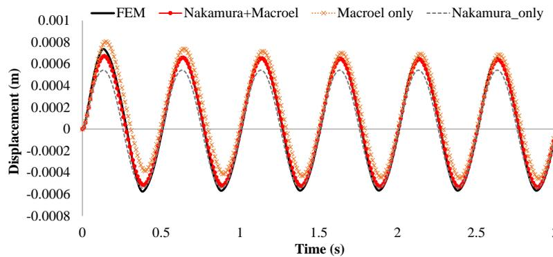
**Fig. 6. Displacement history results for the simplified models and FEM model**
