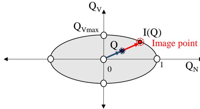
**Fig. 3. Vertical and horizontal bounding surface with current force vector ( $Q$ ) to image point ( $IQ$ )**
