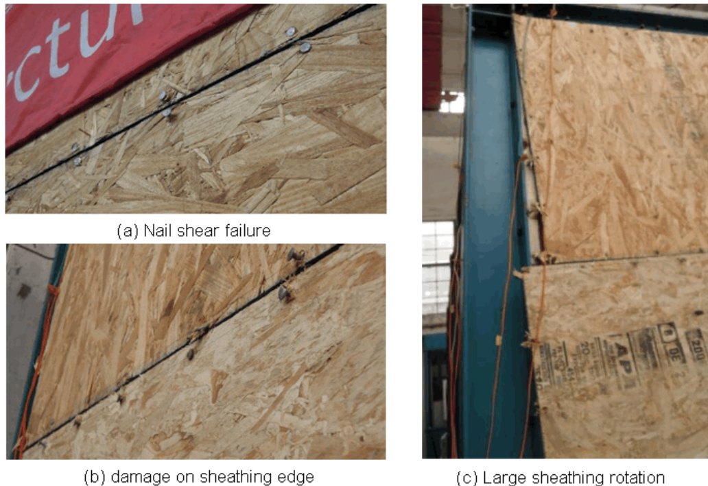
Fig. 1 Damage to timber infill walls during a full-scale testing
